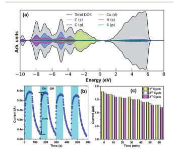
Fig. 8 (a) PDOS analysis of  $Cu_{18}$  NC. (b) Photoresponse properties of the  $Cu_{18}$  NC and (c) their reproducibility.
