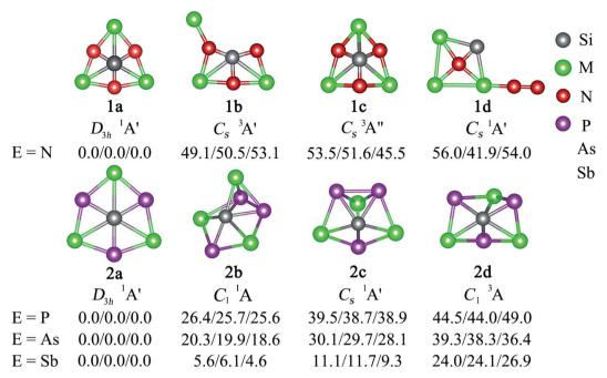
Fig. 2 The structures of low-lying isomers of SiE<sub>x</sub>M<sub>x</sub><sup>+</sup> (E = N, P, As, Sb; M = Ca, Sr, Ba) clusters. Relative energies (in kcal mol<sup>-1</sup>) are shown at the single-point CCSD(T)/def2-TZVP//PBE0/def2-TZVP level, followed by a zero-energy correction at PBE0. The values from left to right refer to Ca, Sr, and Ba in sequence. The group symmetries and electronic states are also given.
