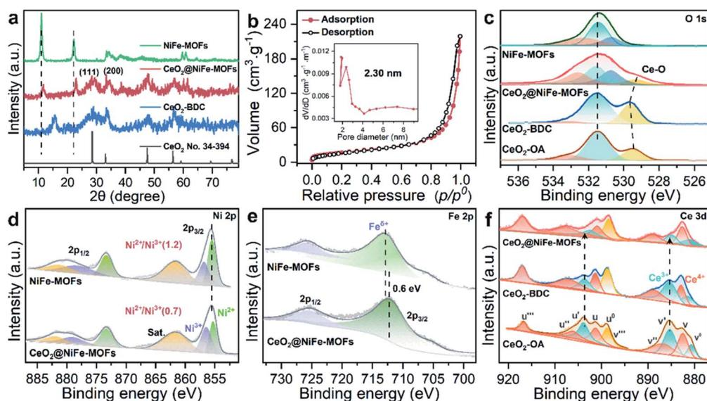
Fig. 2 (a) PXRD patterns of CeO<sub>2</sub> (no. 34–394), CeO<sub>2</sub>-BDC, CeO<sub>2</sub>@NiFe-MOFs and NiFe-MOFs. (b) Nitrogen adsorption/desorption isotherm of CeO<sub>2</sub>@NiFe-MOFs, pore size distributions (inset). (c–f) XPS spectra of O 1s, Ni 2p, Fe 2p and Ce 3d; Ce 3d XPS spectra reveal the change of valence of Ce caused by coordinated functionalization.
