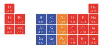
Fig. 8 Initial responses of the electronegativity in a magnetic field as a periodic table representation showing both the numerical values and categorising them with a color code in which blue indicates a positive derivative, red a negative derivative and yellow a derivative that is zero or close to zero.
