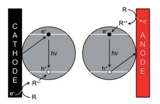
Scheme 1 ECL promotion with QDs. The  $e^-/h^+$  pairs are injected separately by the electrode and the co-reactant, respectively following either the cathodic (left) or anodic ECL pathway (right). Adapted from ref. 181 with permission from the American Chemical Society, Copyright 2014.
