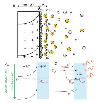
Fig. 3 (a) Scheme of the space charge layer in an n-SC (left) and the Helmholtz layer at the SC/liquid interface (right), adapted with permission from ref. 92  $\phi_{IHL}$  and  $\phi_{OHL}$  are the inner and the outer Helmholtz planes. (b) Scheme showing a depleted n-SC in equilibrium with an electrolyte containing the ox/red redox couple in the dark. (b) Scheme showing the effect of illumination  $(h\nu > E_{\alpha})$  on this junction.
