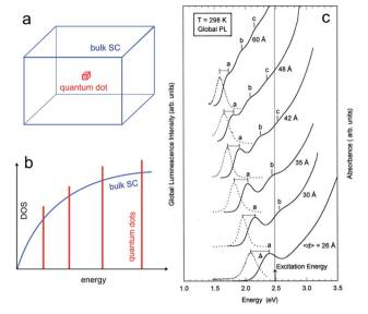
Fig. 2 (a) Scheme showing a 3D bulk SC (blue) and a "0D" quantum dot (red). (b) Density of states (DOS) functions for a bulk SC (blue) and a quantum dot (red). (c) Absorption (solid line) and global PL (dotted line) spectra for InP quantum dots with different mean diameters. The photoexcitation was done at 2.48 eV. Reproduced from ref. 74 with permission from the American Chemical Society, Copyright 1997.
