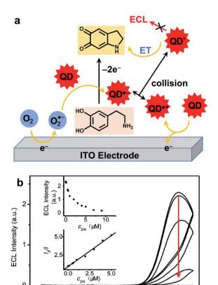
Fig. 10 Detection of catechol with CdTe QDs. (a) Chemical mechanism leading to ECL quenching. (b) ECL curves collected in phosphate buffer without (top curve) and with an increase amount of dopamine (DA, from 50 nM to 50  $\mu$ M) and figures of merit of the sensor (insets). Adapted from ref. 201 with permission from the American Chemical Society, Copyright 2007.
