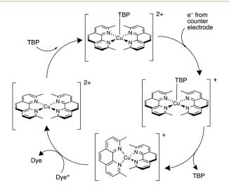
Scheme 7 Representation of the involvement of a strong Lewis base such as TBP in the redox cycle of the [Cu(Me<sub>2</sub>phen)<sub>2</sub>]<sup>2+</sup>/[Cu(Me<sub>2</sub>phen)<sub>2</sub>]<sup>+</sup> mediator. Based on a scheme from the work of Bach and coworkers.119
