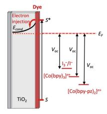
Fig. 3 Schematic illustration of the relative  $E_{\rm redox}$  levels (in red) for two representative  $Co^{3+}/Co^{2+}$  redox mediators with respect to the  $I_3^-/I^$ couple and the effect on the value of  $V_{\rm OC}$  (see Fig. 2a for complete DSC diagram).
