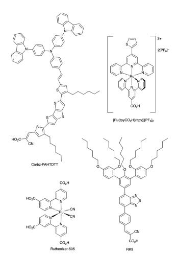
Scheme 12 Structures of the metal-free dyes Carbz-PAHTDTT and RR9, and the ruthenium(II) dyes  $[Ru(tpyCO_2H)(ttpy)][PF_6]_2$  (tpy = 2,2':6',2"-terpyridine) and the commercially available Ruthenizer-505.
