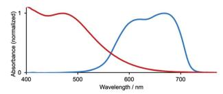
Fig. 10 Solid-state absorption spectra of FTO/ $\text{TiO}_2$  electrodes with adsorbed dyes  $[\text{Cu}(11)(45)]^+$  (red) and SQ2 (blue). The high-energy tail arises from  $\text{TiO}_2$  absorption (spectra recorded by Frederik Malzner, University of Basel).
