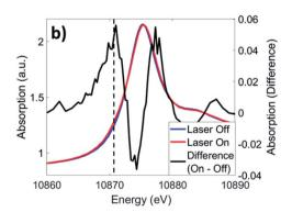
Fig. 4 XTA spectra of CuOs at the (a) Cu K-edge and (b) Os L<sub>III</sub>-edge at 2 ps and 0.7 ps time delays, respectively, following 500 nm excitation. Dotted lines indicate the energies used for kinetics traces in Fig. 5.
