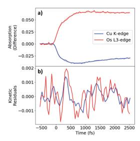
Fig. 5 (a) Kinetics traces for CuOs measured at Cu K (8.986 keV, blue) and Os  $L_{\rm III}$  (10.871 keV, red) edges. Experimental data and fits shown as solid and dotted lines, respectively. (b) Filtered kinetic residuals, with Os residual inverted for comparison.
