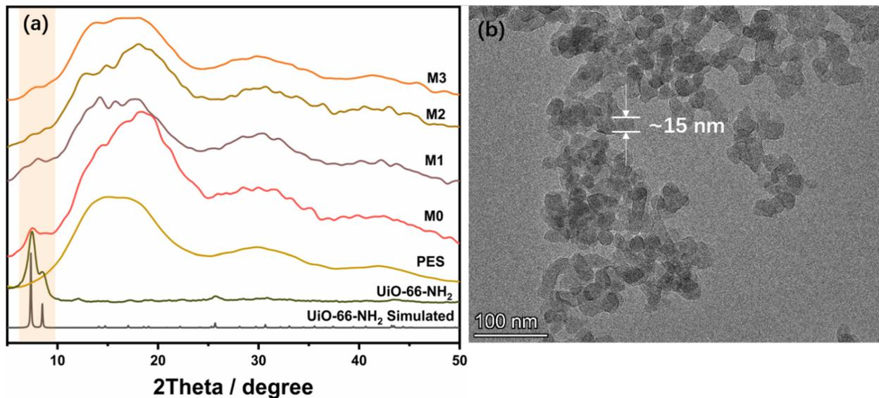
Fig. 3 (a) XRD patterns of UiO-66-NH<sub>2</sub> simulated, UiO-66-NH<sub>2</sub>, PES substrate, and M0–M3. (b) TEM of the L-UiO-66-NH<sub>2</sub>.
