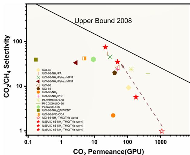
**Fig. 10** Comparison of the  $\text{CO}_2/\text{CH}_4$  separation performances between the IL@UiO-66-NH<sub>2</sub>-TMC membranes prepared in this study and other UiO-66 polycrystalline and composite membranes reported in the literature. Upper bound front drawn assuming a membrane thickness of 1  $\mu\text{m}$ . Detailed information in this figure is listed in Table S3 (ESI†).
