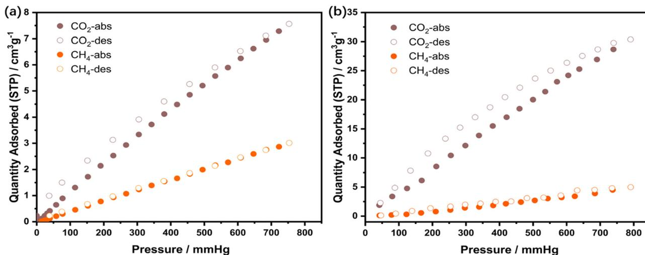
Fig. 7 (a) CO<sub>2</sub> and CH<sub>4</sub> adsorption–desorption isotherms of the M0 membrane at 298 K. (b) CO<sub>2</sub> and CH<sub>4</sub> adsorption–desorption isotherms of M2 membrane at 298 K.
