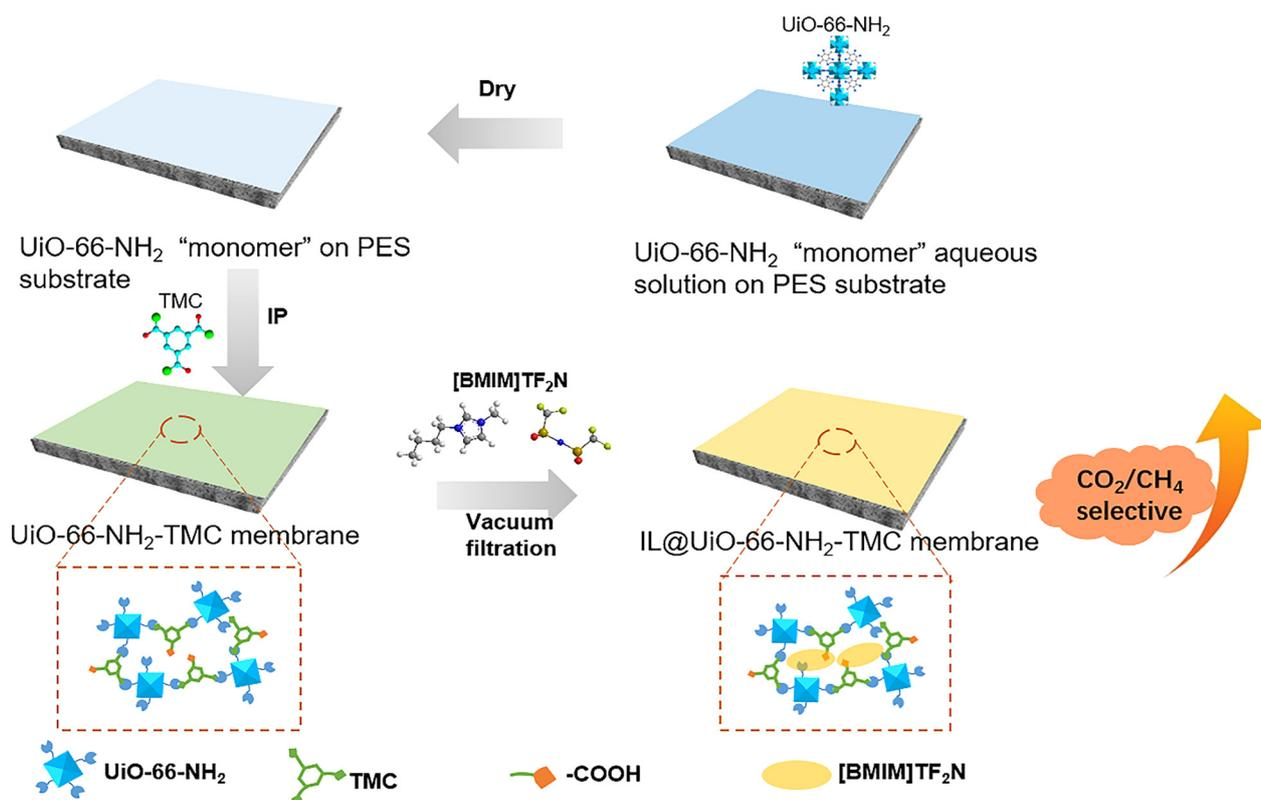
Scheme 1 Preparation of the IL@UiO-66-NH<sub>2</sub>-TMC membrane.
