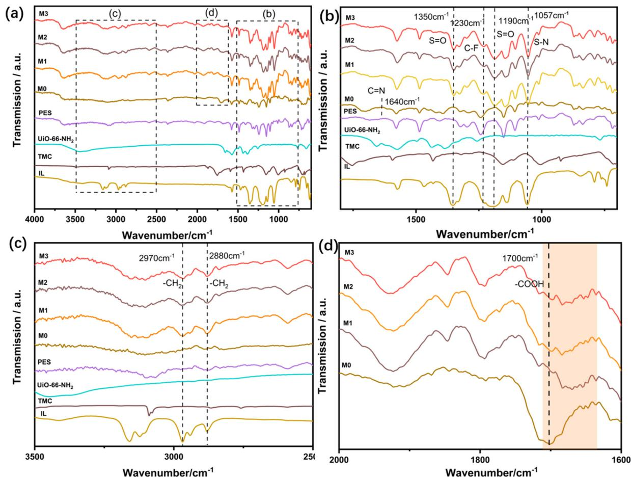
Fig. 1 (a) The FT-IR spectra of IL, TMC, UiO-66-NH<sub>2</sub>, PES substrate, UiO-66-NH<sub>2</sub>-TMC membrane (M0), and IL@UiO-66-NH<sub>2</sub>-TMC membranes prepared with IL concentration of 10 wt%, 15 wt%, and 20 wt% (M1–M3); (b–d) the magnified parts of (b–d) in (a).
