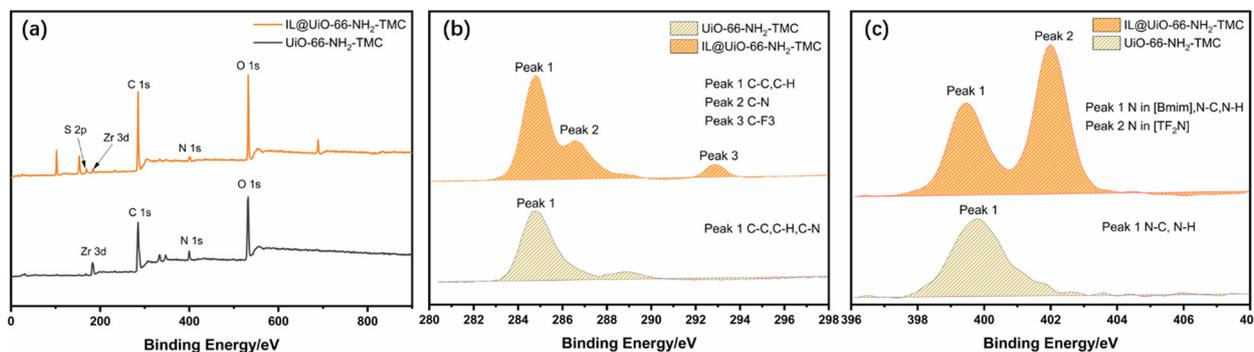
Fig. 2 XPS spectrum of (a) UiO-66-NH<sub>2</sub>-TMC and IL@UiO-66-NH<sub>2</sub>-TMC membranes, (b) C 1s for UiO-66-NH<sub>2</sub>-TMC and IL@UiO-66-NH<sub>2</sub>-TMC membranes, (c) N 1s UiO-66-NH<sub>2</sub>-TMC and IL@UiO-66-NH<sub>2</sub>-TMC membranes.
