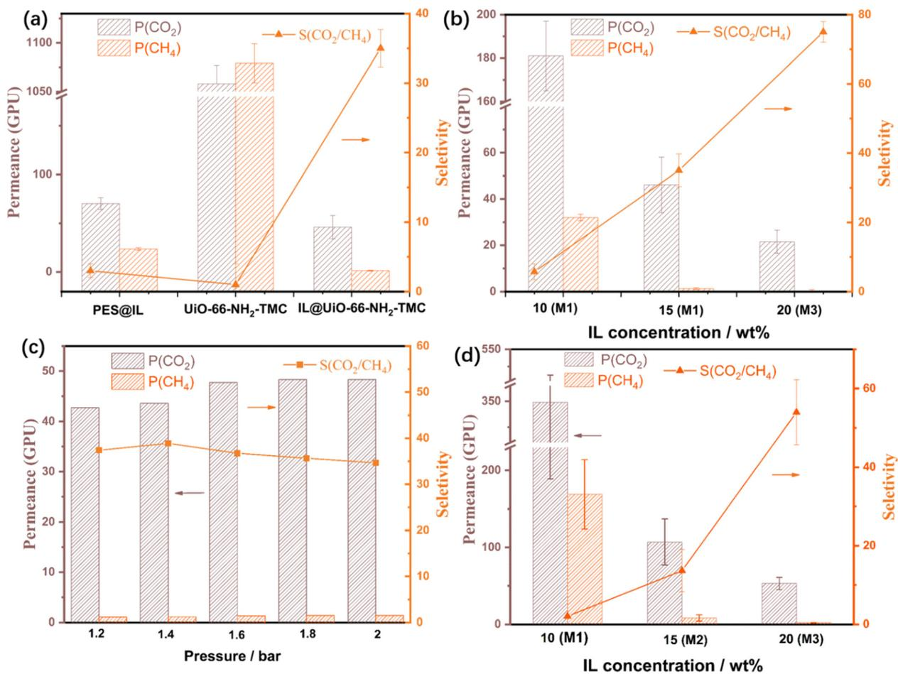
Fig. 8 (a) Mixed gas permeation properties of the PES@IL, UiO-66-NH<sub>2</sub>-TMC, and IL@UiO-66-NH<sub>2</sub>-TMC membrane at 25 °C. (b) Mixed gas permeation properties of the M1–M3 membranes at 25 °C. (c) Mixed gas permeation properties of the M2 membrane under different trans-membrane pressure drops. (d) Single gas permeation properties of the M1–M3 membranes at 25 °C.
