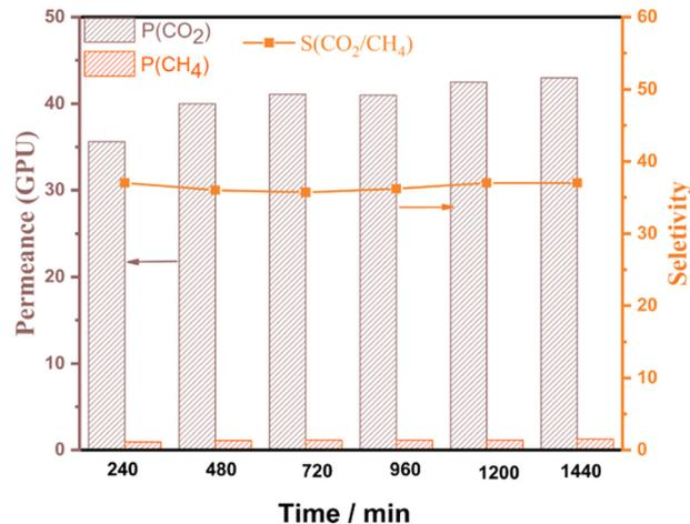
Fig. 9 The plot of CO<sub>2</sub>/CH<sub>4</sub> permeance and selectivity for the IL@UiO-66-NH<sub>2</sub>-TMC membrane versus test time.
