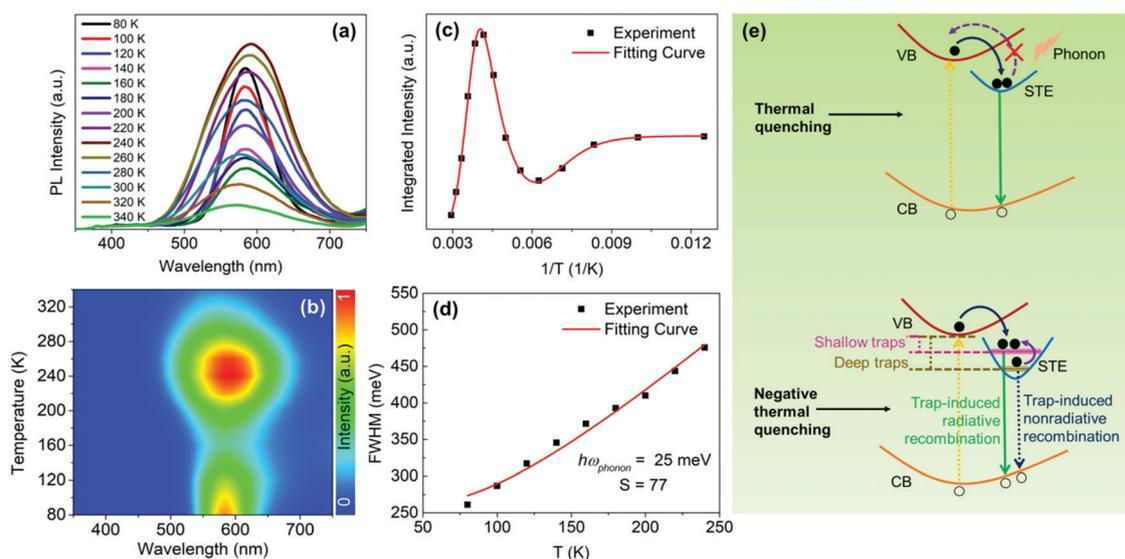
**Fig. 5** (a) Temperature-dependent PL spectra and (b) pseudocolor map of the temperature-dependent PL spectra of  $\text{CsCu}_2\text{I}_3$ . (c) Fitting result of the integrated PL intensity as a function of temperature. (d) Fitting result of the FWHM as a function of temperature. (e) Schematic diagram of thermal quenching and negative thermal quenching processes.
