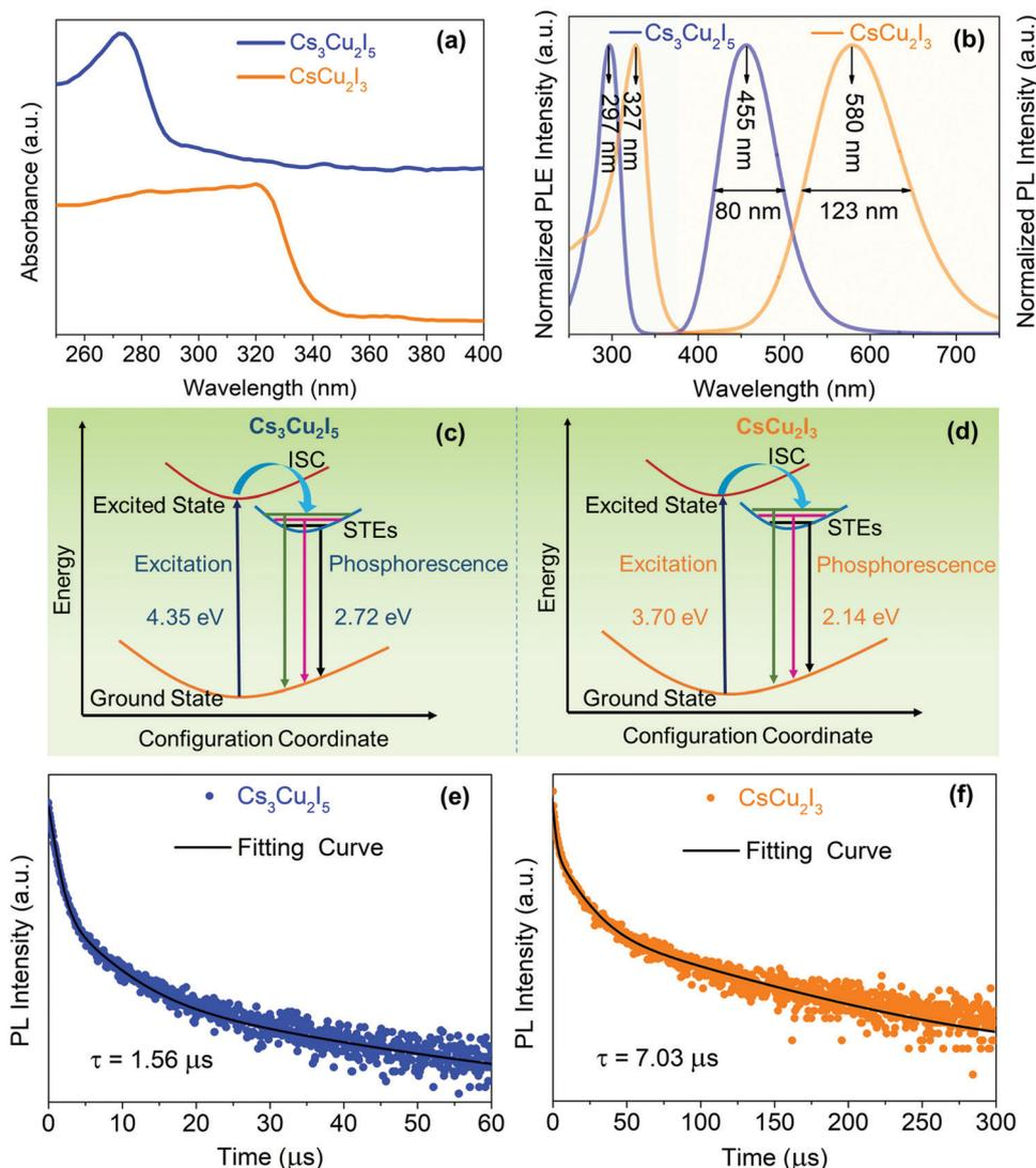
**Fig. 3** (a) UV-vis absorption spectra of  $\text{Cs}_3\text{Cu}_2\text{I}_5$  and  $\text{CsCu}_2\text{I}_3$ . (b) PLE and PL spectra of  $\text{Cs}_3\text{Cu}_2\text{I}_5$  and  $\text{CsCu}_2\text{I}_3$ . Schematic diagram of the STE emission of (c)  $\text{Cs}_3\text{Cu}_2\text{I}_5$  and (d)  $\text{CsCu}_2\text{I}_3$ . Time-resolved PL decay spectra of (e)  $\text{Cs}_3\text{Cu}_2\text{I}_5$  and (f)  $\text{CsCu}_2\text{I}_3$ .
