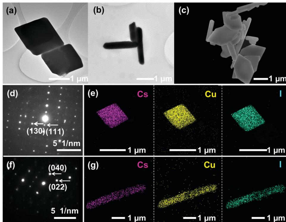
Fig. 2 TEM images of (a)  $\text{Cs}_3\text{Cu}_2\text{I}_5$  and (b)  $\text{CsCu}_2\text{I}_3$ . (c) SEM image of  $\text{CsCu}_2\text{I}_3@ \text{Cs}_3\text{Cu}_2\text{I}_5$  composites. (d) SAED patterns of  $\text{Cs}_3\text{Cu}_2\text{I}_5$ . (e) EDS elemental mapping of Cs, Cu, and I elements in  $\text{Cs}_3\text{Cu}_2\text{I}_5$ . (f) SAED patterns of  $\text{CsCu}_2\text{I}_3$ . (g) EDS elemental mapping of Cs, Cu, and I elements in  $\text{CsCu}_2\text{I}_3$ .
