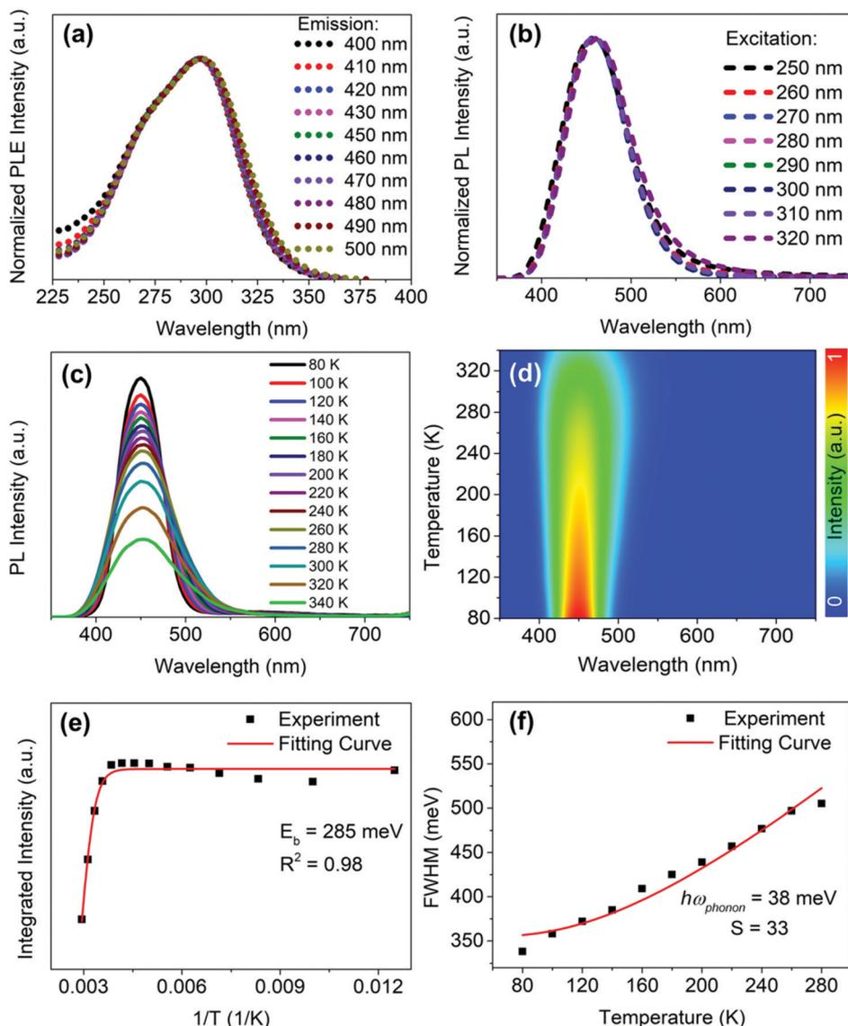
Fig. 4 (a) PLE spectra of  $\text{Cs}_3\text{Cu}_2\text{I}_5$  measured at different emission wavelengths. (b) PL spectra of  $\text{Cs}_3\text{Cu}_2\text{I}_5$  measured at different excitation wavelengths. (c) Temperature-dependent PL spectra and (d) pseudocolor map of the temperature-dependent PL spectra of  $\text{Cs}_3\text{Cu}_2\text{I}_5$ . (e) Fitting result of the integrated PL intensity as a function of temperature. (f) Fitting result of the FWHM as a function of temperature.
