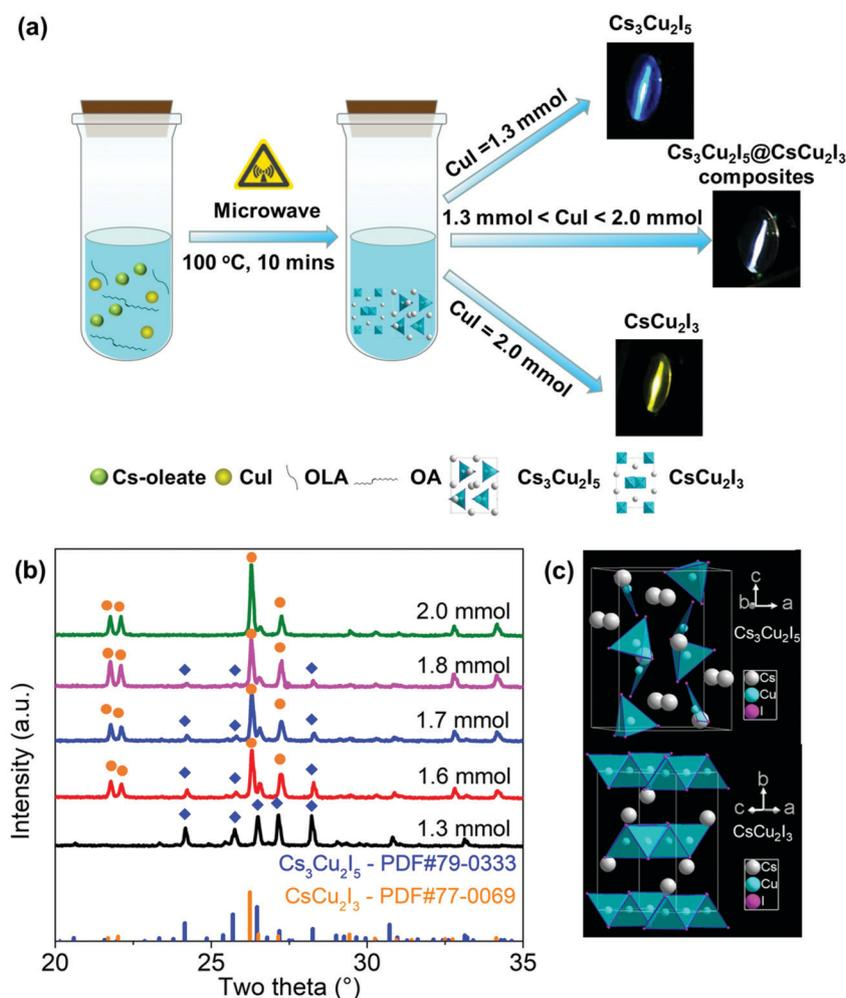
**Fig. 1** (a) Schematic diagram of the microwave synthesis. (b) XRD patterns of samples synthesized with different amounts of CuI. (c) Crystal structures of  $\text{CsCu}_2\text{I}_3$  and  $\text{Cs}_3\text{Cu}_2\text{I}_5$ .
