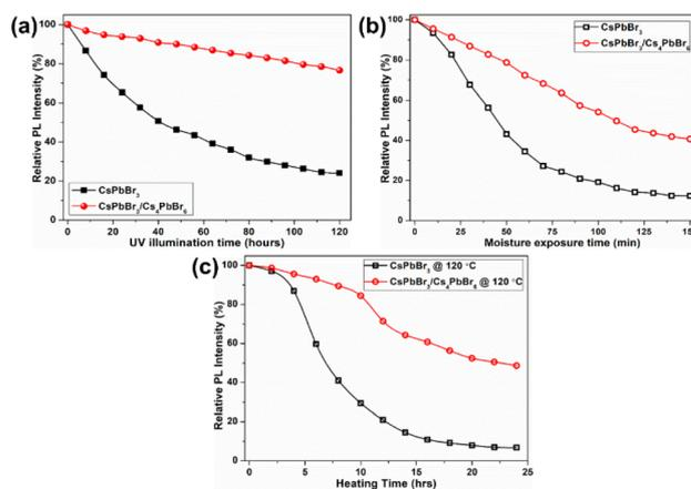
**Fig. 8** (a) UV irradiation test, (b) moisture resistance test, and (c) thermal tolerance test for CsPbBr<sub>3</sub> NCs and dual-phase CsPbBr<sub>3</sub>/Cs<sub>4</sub>PbBr<sub>6</sub> MCs conducted by monitoring their emission trends at 365 nm excitation.
