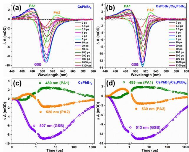
**Fig. 6** Femtosecond transient absorption (fs-TA) spectra of (a) CsPbBr<sub>3</sub>, (b) CsPbBr<sub>3</sub>/Cs<sub>4</sub>PbBr<sub>6</sub> measured for various pump–probe delay times at 400 nm excitation, excited-state kinetic curves for the PA1, GSB, and PA2 of (c) CsPbBr<sub>3</sub>, (d) CsPbBr<sub>3</sub>/Cs<sub>4</sub>PbBr<sub>6</sub>.
