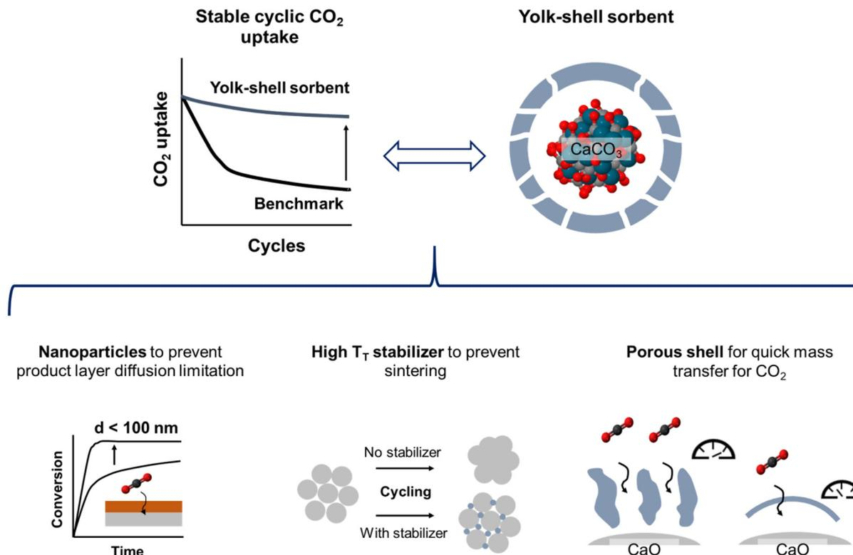
**Fig. 1** Design approach for yolk-shell-type CaO-based sorbents. Using a nanoparticle core is expected to prevent diffusive limitations due to product layer formation, whereas a porous shell of a high  $T_T$  stabilizer shall mitigate sintering of the nanoparticles while at the same time allowing for a rapid transfer of  $\text{CO}_2$  to unreacted CaO.
