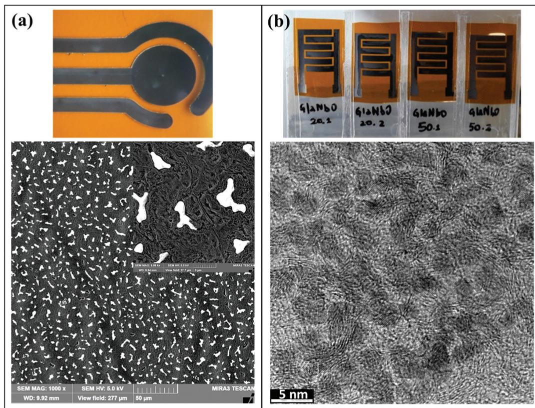
**Fig. 2** (a) Biological electrochemical sensor incorporating gold particles in the active circular region, with the corresponding SEM images showing gold droplets uniformly dispersed in the graphene matrix. The morphology of LIG in a confined environment seems to consist of more densely packed graphene sheets and (b) flexible graphene/ $\text{Nb}_2\text{O}_5$  hybrid MSCs and the corresponding high resolution TEM image showing the nanometric scale oxide grains mixed with the graphene sheets.
