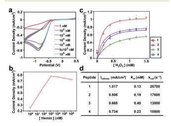
Fig. 3 Electrochemical reduction of  $H_2O_2$  with graphite–peptidehemin hybrid electrodes. (a) Cyclic voltammograms at various concentrations of hemin. (b) The current density of the reduction peak vs. hemin concentration measured in 1 mM  $H_2O_2$  solution. (c) Current density at the reduction peak with various concentrations of  $H_2O_2$  with 1  $\mu$ M hemin. Solid lines show fitting curves with the Michaelis–Menten model. (d) Summary of the kinetic parameters.
