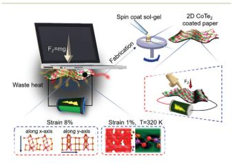
Fig. 1 Schematic representation of the utilization of waste heat by generating electricity and the energy harvesting concept of piezo-tribo generators using 2D CoTe<sub>2</sub>.
