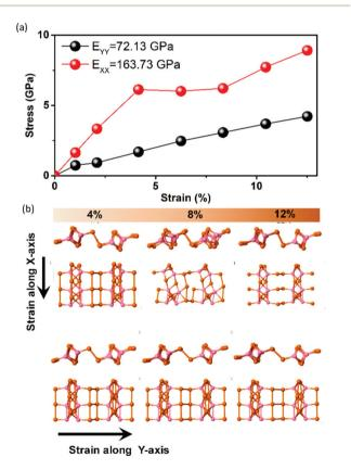
Fig. 5 (a) Stress-strain curves of 2D  $CoTe_2$  considering one supercell composed of 36 atoms. The Young's modulus values for each direction are 163.73 and 72.13 GPa along the X and Y directions, respectively. (b) Deformation of the lattice structure along the X and Y axes as a function of applied strain.
