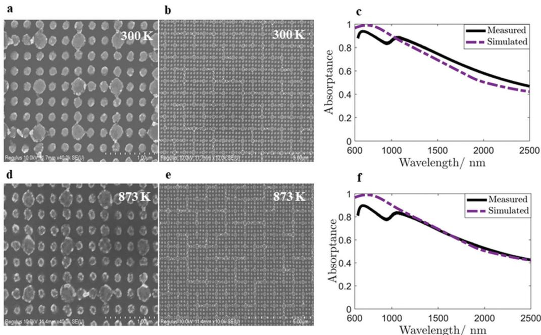
**Fig. 3** SEM images of the absorber and the measured absorbance (a) at 300 K with a scale bar of 1  $\mu\text{m}$  and (b) at 300 K with a scale bar of 5  $\mu\text{m}$ . (c) Comparison of the measured and simulated emittances at 300 K, (d) at 873 K with a scale bar of 1  $\mu\text{m}$ , and (e) at 873 K with a scale bar of 5  $\mu\text{m}$ . (f) Comparison of the measured and simulated emittances at 873 K.
