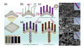
Fig. 8 (a-e) Schematic illustrations of the synthesis of yolk-shell Ni-Mo-Co-S NCAs on NF. SEM images of (f) NiMoO<sub>4</sub>·xH<sub>2</sub>O@ZIF-67, (g) hollow NiMoO<sub>4</sub>·xH<sub>2</sub>O@Ni-Co-S NCAs and (h) yolk-shell Ni-Mo-Co-S NCAs. Reprinted with permission from ref. 98, Copyright 2020, Elsevier.
