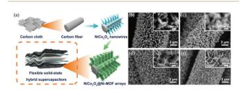
Fig. 4 (a) Schematic illustration of the synthesis of NiCo<sub>2</sub>O<sub>4</sub>@Ni-MOF on CF. (b-e) SEM images of NiCo<sub>2</sub>O<sub>4</sub>@Ni-MOF synthesized at 3, 6, 12, and 24 h for MOF growth, respectively. Reprinted with permission from ref. 58, Copyright 2019, American Chemical Society.
