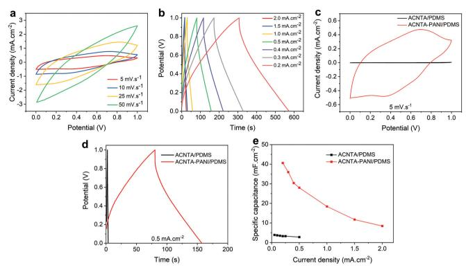
Fig. 5 Electrochemical performance of symmetric two-electrode supercapacitors. (a) CV curves of ACNTA-PANI/PDMS at scan rates varying between 5 and 50 mV s<sup>-1</sup>. (b) GCD curves at different current densities. (c) CV curves of ACNTA/PDMS and ACNTA-PANI/PDMS at a scan rate of 5 mV s<sup>-1</sup>. (d) GCD curves of ACNTA/PDMS and ACNTA-PANI/PDMS at 0.5 mA cm<sup>-2</sup>. (e) Areal specific capacitances calculated for different current densities.
