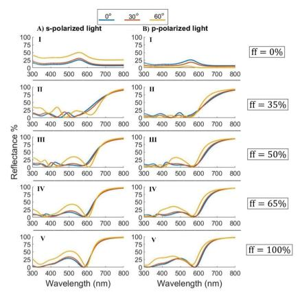
Fig. 6 Reflectance profile for a nanosheet HMM of different metal fractions with different angles of incidence. Color coding of curves correspond to indicated angles of incidence in the top box of the figure. Curves calculated for a hexagonal NP array above a Aq/TiO2 multilayer HMM stack, with all other parameters as in Fig. 4, for the Ag fill fraction as indicated in each panel.
