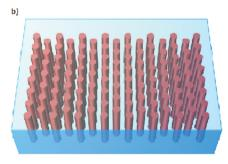
Fig. 1 Most common HMM structures used in theoretical investigations: (a) stacked nanosheet structure and (b) embedded nanowire structure. The former is being considered in the present work.
