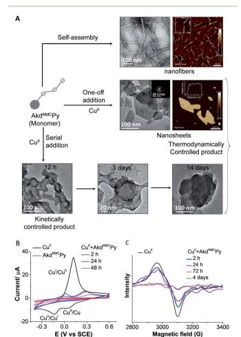
Fig. 3 (A) Differential morphologies of Akd<sup>NMC</sup>Py in the absence and presence of Cu<sup>II</sup>. Akd<sup>NMC</sup>Py self-assembles to form nanofibers. One-off addition of Cu<sup>II</sup> produced 2D nanosheets (inset: SAED pattern of the sheets), while serial addition formed sheets through intermediate micelle-like core-shell architectures. (B and C) CV and EPR spectra of Akd<sup>NMC</sup>Py and Cu<sup>II</sup>, and their complex at various time intervals.
