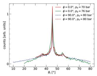
Fig. 1 Angular distribution curves of the bilayer silica film with nanoscale holes supported on Ru(0001). Taken with a beam energy of  $E_i$  = 28.8 meV.  $\phi$  = 0.0° corresponds to the  $\Gamma M$  direction of the substrate. The two curves labelled with  $\phi = 90.0^{\circ}$  are independent runs.
