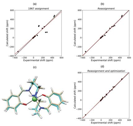
Agreement between experimental and QC calculated shifts of NiSAL-HDPT, with the assignment previously reported (a), $^{124}$  and the theory-based reassignment (b). Comparison between initial (beige) and DFT-optimized (cyan) structures (c) and agreement between the experimental and QC calculated shifts for the refined structure (d).
