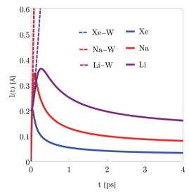
Fig. 2 Time dependence of the coherence length *l*(*t*) for three adsorbates Xe, Li and Na. The initial parameters for the Gaussian wave packet (9) are: position  $x_0 = 0$ , width  $\sigma_0 = 0.003$ (Xe), 0.02(Na) and 0.2(Li) a.u., and momentum  $p_0$  = 0, a temperature T = 105 K and a friction coefficient  $\gamma = 0.25 \text{ ps}^{-1}$ . With environment (solid lines) and without (dashed line): Xe (blue), Na (red) and Li (purple).
