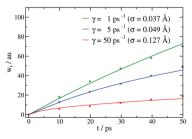
Fig. 10 Time dependence of the wave packet width for Xe adsorbates and different values of  $\gamma$  and  $\sigma$  up to 50 ps. The surface temperature is T = 121 K. The numerical and analytic results are shown by points and solid curves:  $\gamma = 1 \text{ ps}^{-1}$  and  $\sigma = 0.7 \text{ a.u.}$  (green line),  $\gamma = 5 \text{ ps}^{-1}$  and  $\sigma = 0.1 \text{ a.u.}$ (blue line) and  $\gamma = 50 \text{ ps}^{-1}$  and  $\sigma = 0.25 \text{ a.u.}$  (red line).
