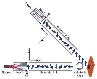
Fig. 1 Schematic of the experimental apparatus showing the positions of the various magnetic elements that are used to manipulate the magnetic moments of the D2 molecules (represented as arrows) and the frames of reference for propagation down the first and second arm of the machine. Hex1. Dip1/Hex2. Dip2 mark the positions of the first/second hexapole magnets and the dipolar fields positioned after/before the hexapoles.
