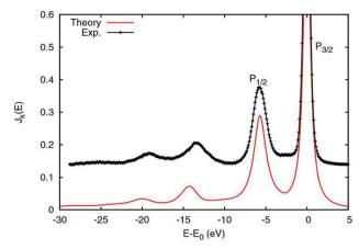
Fig. 9 2p core-level XPS of rutile TiO2 calculated with the real-time cumulant approach (red solid) compared to experimental results (black). The main quasiparticle peaks are labeled  $P_{1/2}$  and  $P_{3/2}$ , while the charge transfer satellites appear at  $\sim 14$  eV lower energy. Reprinted figure with permission from [J. J. Kas, F. D. Vila, J. J. Rehr and S. A. Chambers, Phys. Rev. B, 2015, 91, 121112], Copyright (2022) by the American Physical Society
