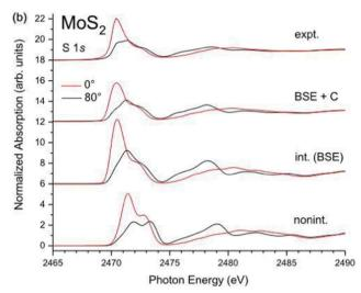
Fig. 11 K-Edge XAS of MoS<sub>2</sub> calculated within the non-interacting approximation (bottom), BSE (second curves), and BSE + cumulant (third curves), compared to experiment (top). The angle of polarization is shown by the colors. Reprinted figure with permission from [J. C. Woicik, C. Weiland, A. K. Rumaiz, M. T. Brumbach, J. M. Ablett, E. L. Shirley, J. J. Kas and J. J. Rehr, Phys. Rev. B, 2020, 101, 245105], Copyright (2022) by the American Physical Society.
