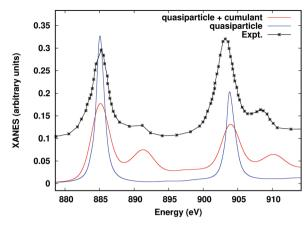
Fig. 14 Ce M-edge XANES of CeO<sub>2</sub> including the many-body convolution with the cumulant spectral function compared to the quasiparticle spectrum and experiment.88
