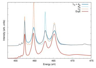
Fig. 8 The Ti L<sub>2.3</sub> edge of SrTiO<sub>3</sub> calculated using three different broadening methods compared to measured data taken from ref. 70. All calculated spectra have a uniform broadening of 0.25 eV full-width at half maximum. Selectively, peaks associated with the  $L_2$  edge ( $2p_{1/2}$  holes) are broadened to 0.52 eV, and peaks associated with the 3d e<sub>a</sub> states are broadened by an additional 0.5 eV.
