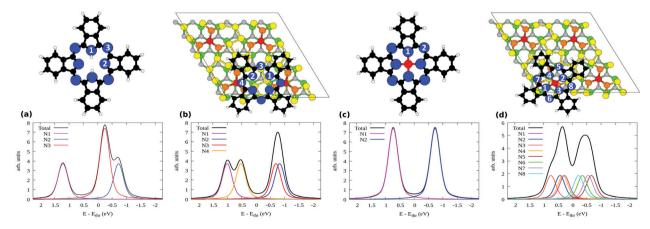
Fig. 8 Simulated N 1s XPS of (a)  $H_2Pc$  molecules, (b) bridge  $H_2Pc/6H-SiC(0001)-(3\times3)$ , (c) SiPc, and (d) top SiPc/6H-SiC(0001)-(3×3). The inequivalent N atoms are numbered in the respective geometries shown above each plot. Refer to Fig. 7 for the color coding used here.
