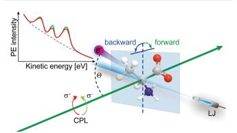
Fig. 7 Depiction of the liquid-jet PECD experiment with backward electron detection relative to the light propagation (green arrow); CPL denotes circularly polarized light. Inset: Fictive carbon 1s PECD spectrum on top of the LET. Illustrated intensity differences correspond to measurements with left- and right-CPL from the same enantiomer in water
