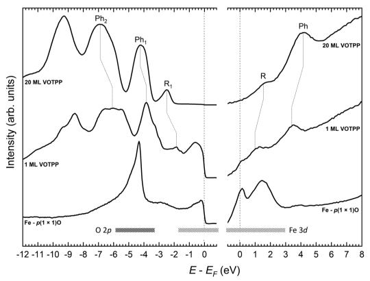
Fig. 2 UPS (left) and IPES (right) spectra acquired on the Fe- $p(1 \times 1)$ O substrate and after the growth of 1 and 20 ML thick VOTPP layers. Photoemission features from O and Fe species are highlighted in the substrate spectra, while labels (R) and (Ph) account for photoemission from the VOTPP macrocycle and peripheral phenyl groups, respectively
