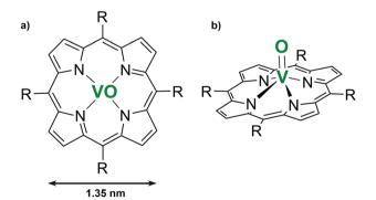
Fig. 1 Schematic representation of a vanadyl-tetraphenyl porphyrin (R = phenyl group). (a) Top view; (b) 3D perspective view highlighting the orientation of the V-O bond along a direction perpendicular to the plane of the tetrapyrrolic ring.
