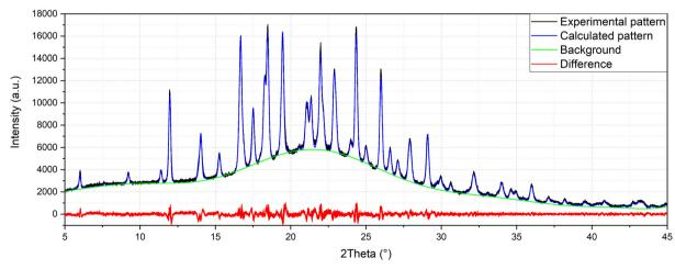
Fig. 3 Comparison of powder patterns of  $1\alpha$  and  $1\beta$  and refinement of crystal structure solved by powder diffraction of  $1\beta$  ( $R_p = 2.043$ ,  $R_{wp} = 1.043$ ). 2.635).
