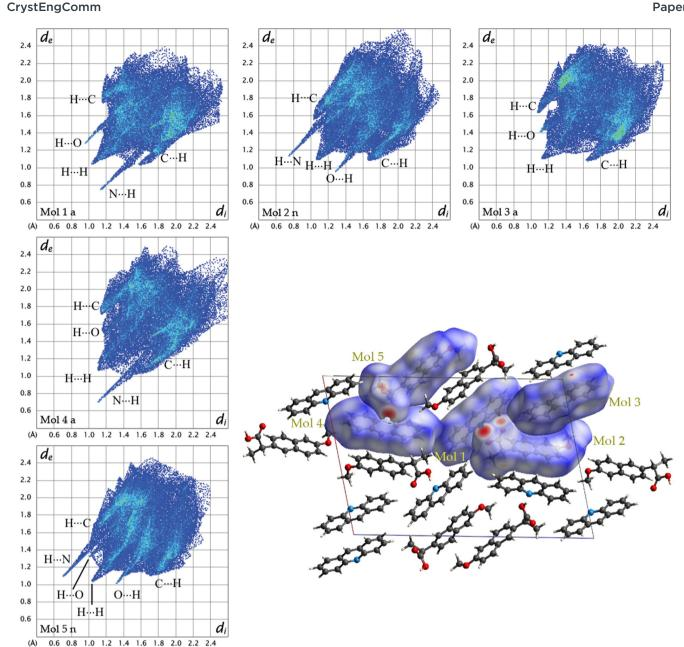
Fig. 6 Fingerprint plots for each symmetry-independent molecule in  $1\alpha$  and crystal structure model of 1a viewed along the b-axis showing Hirshfeld surfaces with d-norm plotted.
