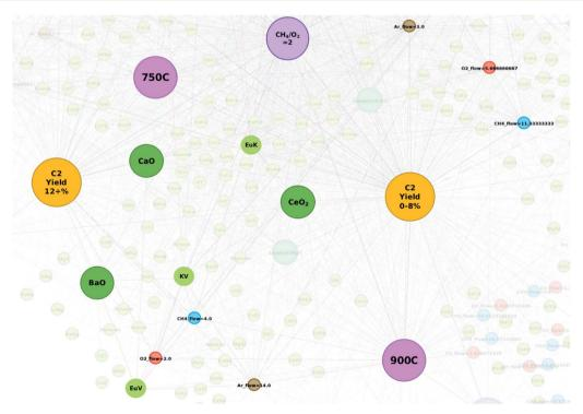
Element pair nodes for proposed catalyst KVEu-BaO and experimental condition nodes that they relate to.
