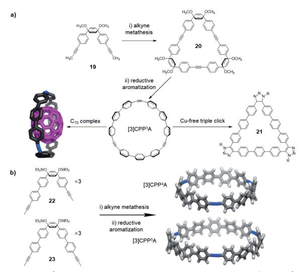
Fig. 6 (a) Synthesis of [3]CPP $^3$ A, and its binding with C $_{70}$  and occurring triple-click reaction. (b) Synthesis of [3]CPP $^4$ A and [3]CPP $^5$ A structures. Reproduced with permission: (a) from ref. 59, Copyright 2016, The American Chemical Society; (b) from ref. 60, Copyright 2019, The American Chemical Society.
