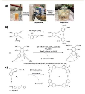
Fig. 2 Representative driving-force in alkyne metathesis: (a) evaporation-driven; (b) adsorption-driven; (c) precipitate-driven. Reproduced with permission: (a) from ref. 36, Copyright 2021, Springer Nature; (b) from ref. 38, Copyright 2013, Wiley; from ref. 39, Copyright 2020, The Royal Society of Chemistry; (c) from ref. 41, Copyright 2004, The American Chemical Society.
