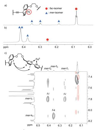
Fig. 2 (a and b)  $^1$ H NMR spectra of [2bFe](PF<sub>6</sub>)<sub>2</sub> (600 MHz, 5.9–6.5 ppm). (a) CD<sub>3</sub>CN. (b) CDCl<sub>3</sub>. (c)  $^1$ H $^-$ 1H ROESY spectrum of [2bFe](TFPB)<sub>2</sub>. See Fig. S47† for the detailed assignment of the signals. The characteristic ROE correlations supporting the structure of *mer*-[2bFe](TFPB)<sub>2</sub> are highlighted (signals of the *mer*-isomer are numbered for each tripodal arm).
