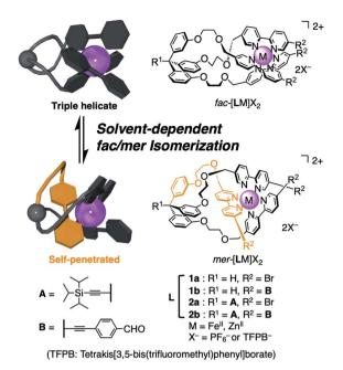
Fig. 1 Schematic representations of the interconversion between the facial (fac) and meridional (mer) isomers and chemical structures of both isomers of  $[LM]X_2$  (L: tripodal ligands (1a, 1b, 2a, and 2b); M: octahedral metal; X: anion).
