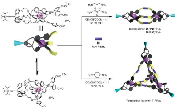
Fig. 6 Bicyclic dimer D-PPD<sup>4+</sup> and D-CHZ<sup>4+</sup>, and tetrahedral tetramer  $T^{8+}$ , which are constructed by the imine bond formation of  $[2bFe]^{2+}$  existing as a fac/mer isomeric mixture.
