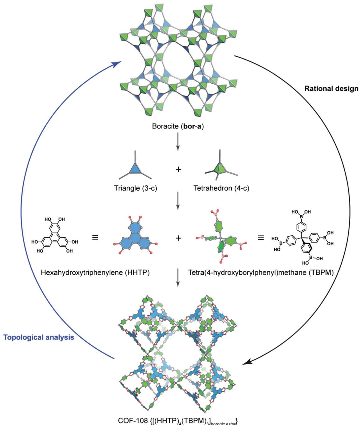
Fig. 3 Reticular design of the augmented boracite topology (**bor-a**) which is deconstructed into triangles (3-c) and tetrahedra (4-c) corresponding to HHTP and tetra(4-hydroxyborylphenyl)methane (TBPM), respectively. TBPM reacts with HHTP to form COF-108  $\{[(\text{HHTP})_4(\text{TBPM})_3]_{\text{boronic ester}}\}$ . The opposite way of rational design is the topological analysis.
