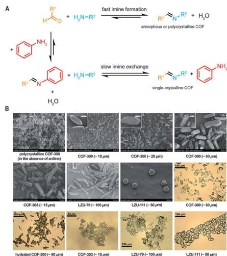
**Fig. 8** Comparison between fast imine condensation (in the absence of aniline) and slow imine condensation (in the presence of aniline) reaction (A). The slow imine exchange enables the formation of single crystals of 3D imine-based COFs (B). Reproduced with permission.<sup>44</sup> Copyright 2018, American Association for the Advancement of Science.
