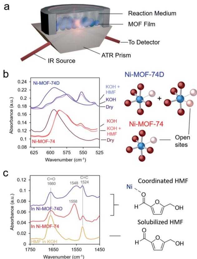
Fig. 3 An ATR configuration was used to probe the MOF-HMF interactions (a). The low wavenumber spectra reveal that Ni-MOF-74D has more open coordination sites in which OH can adsorb, which is then partially displaced by HMF (b). The HMF-Ni interactions can also be visualized in the high wavenumber region in which a new band arises, stemming from the interaction of the HMF aldehyde group with the Ni centers of the MOFs (c).
