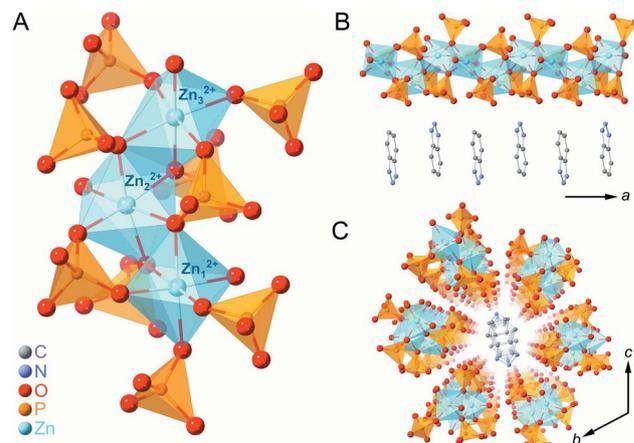
Fig. 1 (A) Local coordination geometry in **1a**. (B) Crystal structure of the one-dimensional (1D) chain along the *a*-axis. (C) Packing structure of **1a** on the *bc*-plane. Zn, P, O, C, and N atoms are represented by light blue, orange, red, grey, and blue spheres, respectively. H atoms are omitted for clarity.
