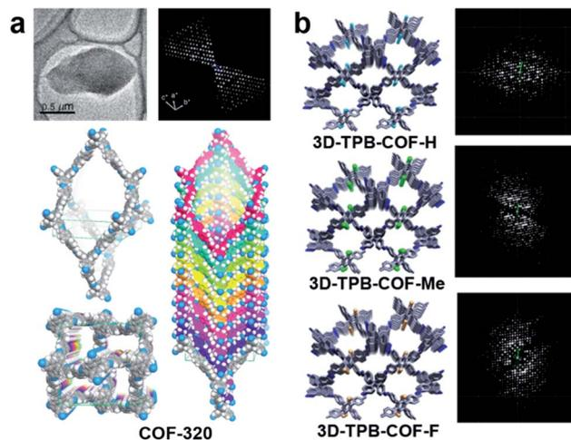
Fig. 12 (a) COF-320, with different structures at 298 K and 89 K, which were both determined by RED.<sup>98</sup> (b) A series of 3D-TPB-COFs, whose structures were determined by cRED.<sup>99</sup> Reproduced from ref. 98 and 99 with permission from the American Chemical Society, and the John Wiley & Sons, Inc., respectively copyright 2013 and 2019.
