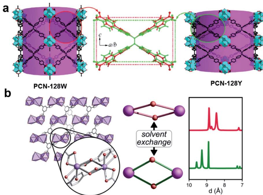
Fig. 10 Illustration of structural changes in flexible MOFs (a) PCN-128<sup>74</sup> and (b) SU-100,<sup>81</sup> whose structures are revealed by 3DED. Reproduced from ref. 74 and 81 with permission from the American Chemical Society, copyright 2015 and 2019.
