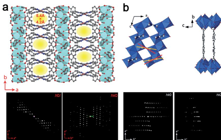
Fig. 9 Structural models and corresponding cRED data of (a) PCN-226, a Zr-oxo chain based structure,<sup>84</sup> and (b) COK-47, a Ti-oxo sheet based structure.<sup>82</sup> All of them are obtained as nanocrystals, and the structures are determined using cRED data. Reproduced from ref. 82 and 84 with permission from the American Chemical Society, and John Wiley & Sons, Inc., respectively, copyright 2020 and 2019.
