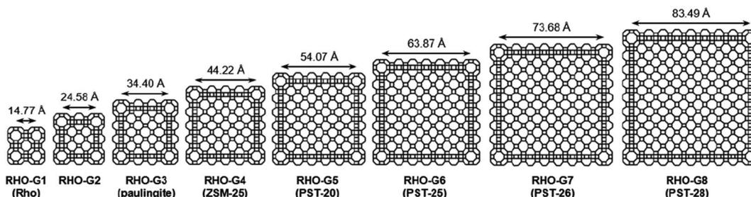
Fig. 6 Framework representations of cross sections (ca. 12 Å thick) of RHO-G1 to RHO-G8 in the RHO family of embedded isorecticular zeolites.<sup>66</sup> Reproduced from ref. 66 with permission from the John Wiley & Sons, Inc., copyright 2016.
