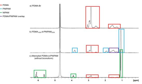
Fig. 3 <sup>1</sup>H NMR spectrum showing (a) PDMA-Br after precipitation, (b) PDMA<sub>1500</sub>-b-PNIPAM<sub>3330</sub> (using 2 mol% bromoform in step 1) after precipitation and (c) only NIPAM monomer peaks present for the attempted synthesis of PDMA-b-PNIPAM from PDMA (0 mol% bromoform in step 1).
