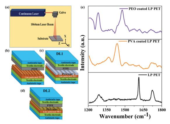
Fig. 1 (a) Schematic diagram of laser processing (b) pristine LP-PTFE TENG device, (c) PVA coated LP-PTFE TENG, (d) PEO coated LP-PTFE TENG device, and (e) Raman shift before and after PEO/PVA coating of the LP PET surface.
