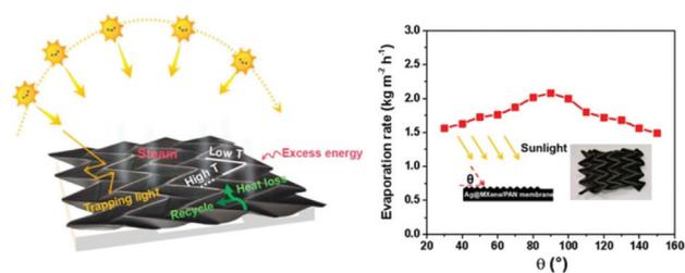
**Fig. 7** Improvement of energy efficiency. Schematic illustration of an origami-structured evaporator and evaporation rate under incident light with different incident angles. This figure has been reproduced from ref. 46 with permission from Elsevier, copyright 2021.
