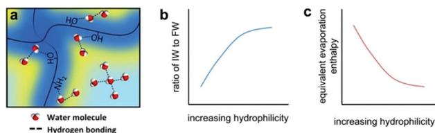
**Fig. 6** Enhancing evaporation by decreasing the vaporization enthalpy of water. Schematic illustration of the (a) water state, (b) intermediate water ratio, and (c) equivalent evaporation enthalpy of water in a hydrogel. This figure has been reproduced from ref. 37 with permission from American Association for the Advancement of Science, copyright 2019.
