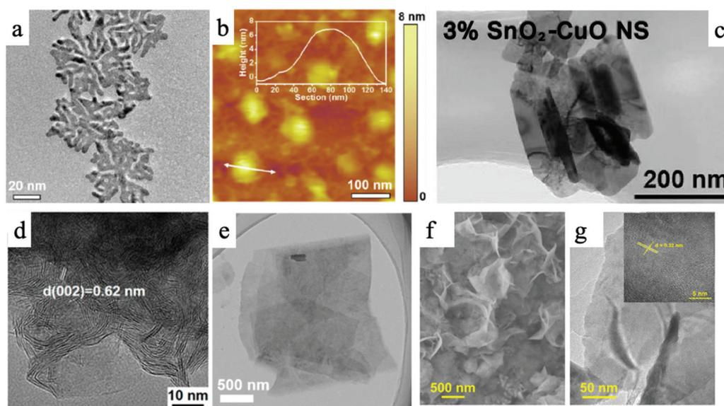
**Fig. 1** An overview of different types of 2D materials. (a) and (b) TEM and AFM images of 2D palladium-copper alloy nanodendrites; (c) SnO<sub>2</sub> modified two-dimensional CuO nanosheet; (d) TEM image of MoS<sub>2</sub> nanosheet; (e) TEM image of Ultrathin 2D Mxene. (f) and (g) TEM images of Bi-MOF ultrathin nanosheet.<sup>30–34</sup>
