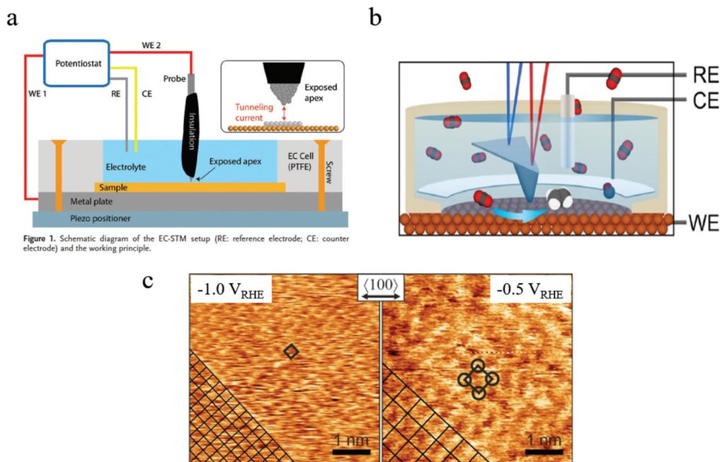
Fig. 5 (a) Schematic of *in situ* EC-STM setup. Copyright 2018, John Wiley and Sons; (b) schematic of *in situ* EC-AFM; (c) morphology of Cu surface at different potentials characterized by *in situ* AFM. Copyright 2020, John Wiley and Sons. All panels reproduced with permission.<sup>139,143</sup>
