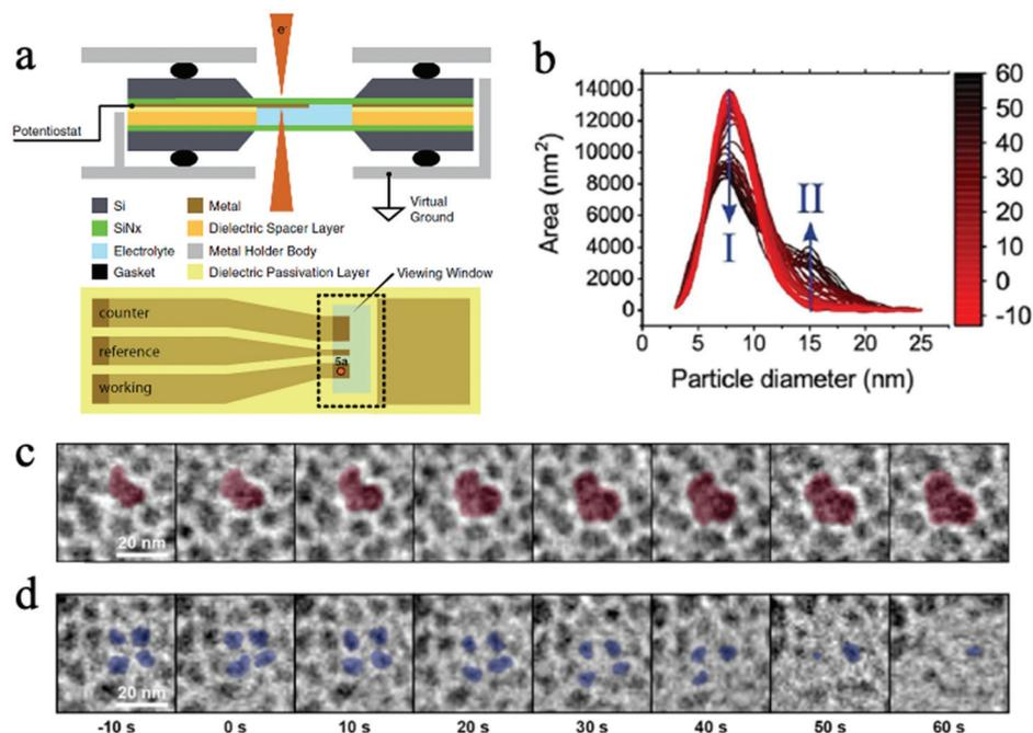
**Fig. 6** (a) The schematic of a micro electrochemical cell for *in situ* TEM. Copyright 2017, IOP Publishing, Inc.; (b) the change in primary (I) and secondary (II) particle sizes as experiment progresses; (c) the growth of secondary particles, and (d) the shrinkage of primary particles. Copyright 2020, John Wiley and Sons. All panels reproduced with permission.<sup>152,154</sup>
