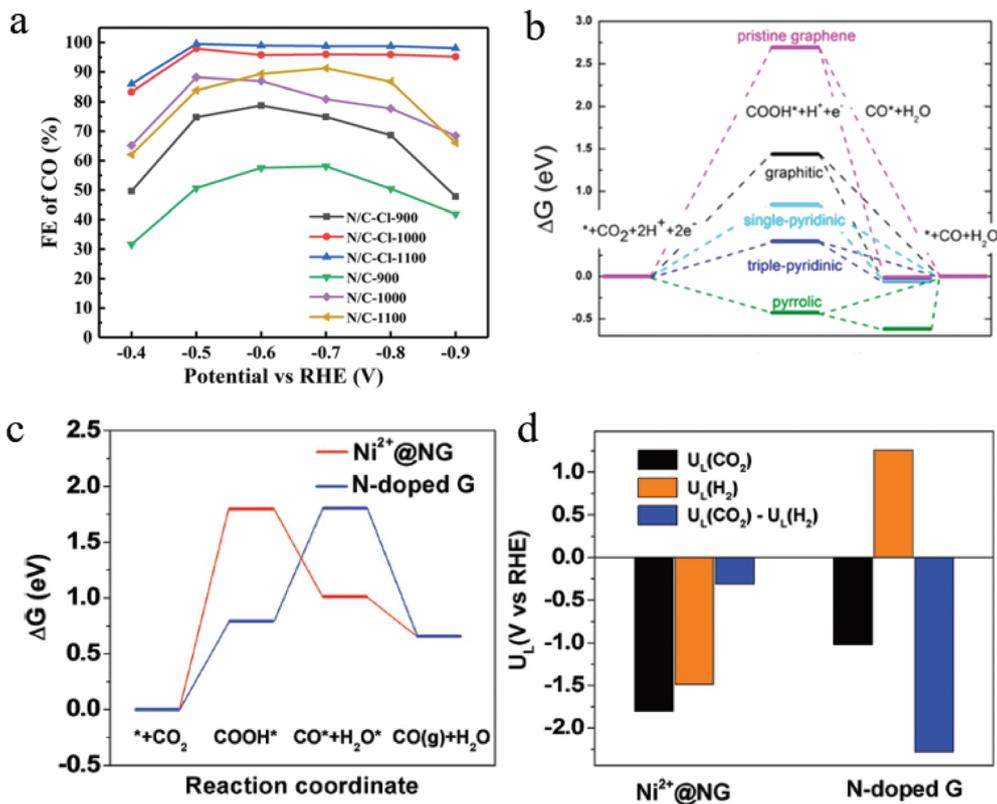
**Fig. 2** (a) FE of catalysts with different surface areas. Copyright 2021, Springer Nature; (b) free energy diagram of CO<sub>2</sub> ECR to CO on different NG surfaces. Copyright 2016, American Chemical Society; (c) free energy diagrams and (d) the calculated limiting potentials for CO<sub>2</sub>RR and HER on composite and pristine graphene surfaces. Copyright 2018, John Wiley and Sons. All panels reproduced with permission.<sup>23,92,96</sup>
