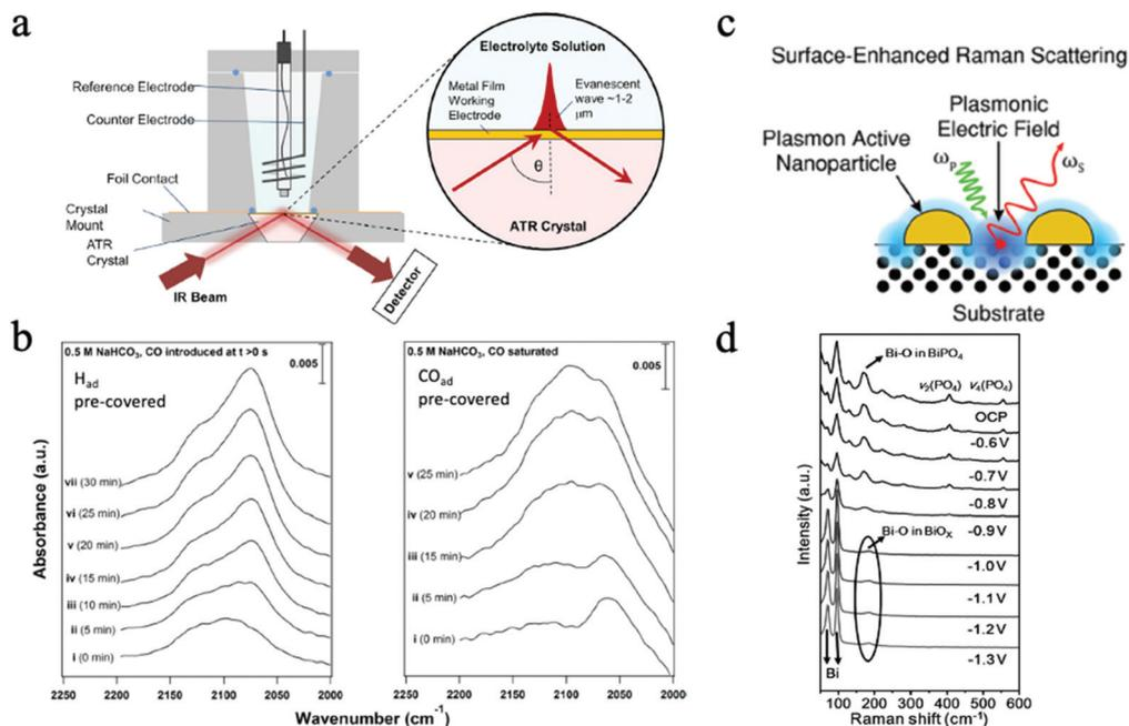
**Fig. 10** (a) Mechanism of *in situ* ATR. Copyright 2017, crown; (b) time-resolved SEIRA spectra of H<sub>ad</sub> accumulation on CO-adsorbed Cu surface. Copyright 2016, American Chemical Society (c) mechanism of SERS. Copyright 2021, Royal Society of Chemistry; (d) *operando* Raman spectra under different applied potential. All panels reproduced with permission.<sup>198–201</sup> Copyright 2021, 2021 Wiley and Sons.
