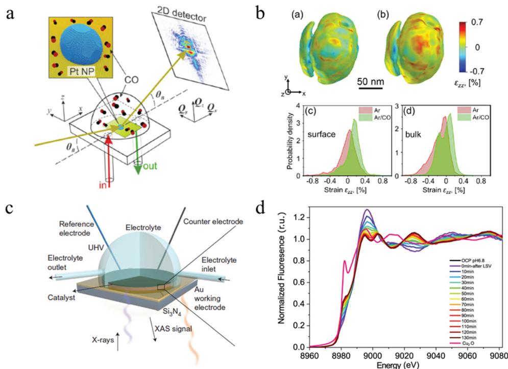
**Fig. 8** (a) The schematic of CXDI imaging. (b) 3D CXDI imaging of Pt NP under different conditions and the strain field in near surface region and in the bulk. Copyright 2019, American Chemical Society; (c) *in situ* XAS electrochemical cell. Copyright 2017, Springer Nature; (d) time-resolved XAS spectrum. Copyright 2021, Springer Nature. All panels reproduced with permission.<sup>153,164,171</sup>
