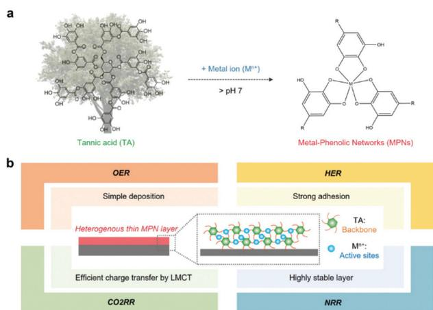
**Fig. 1** (a) Schematic illustration of the formation of metal–phenolic networks (MPNs) in the presence of tannic acid and metal ions. (b) Properties of heterogeneous thin MPN films and their application in various electrochemical reactions.
