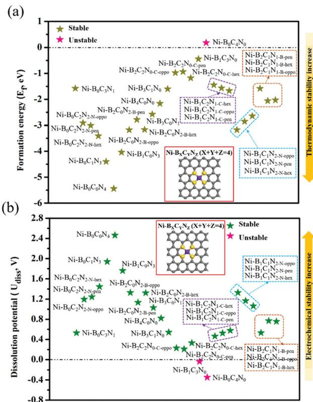
**Fig. 1** The DFT-computed formation energy (a) and dissolution potential (b) of Ni–B<sub>*X*</sub>C<sub>*Y*</sub>N<sub>*Z*</sub> (*X* + *Y* + *Z* = 4). The inset shows the top view of the catalyst model, where the highlighted yellow atoms represent the coordination atoms of the Ni center (purple atom).
