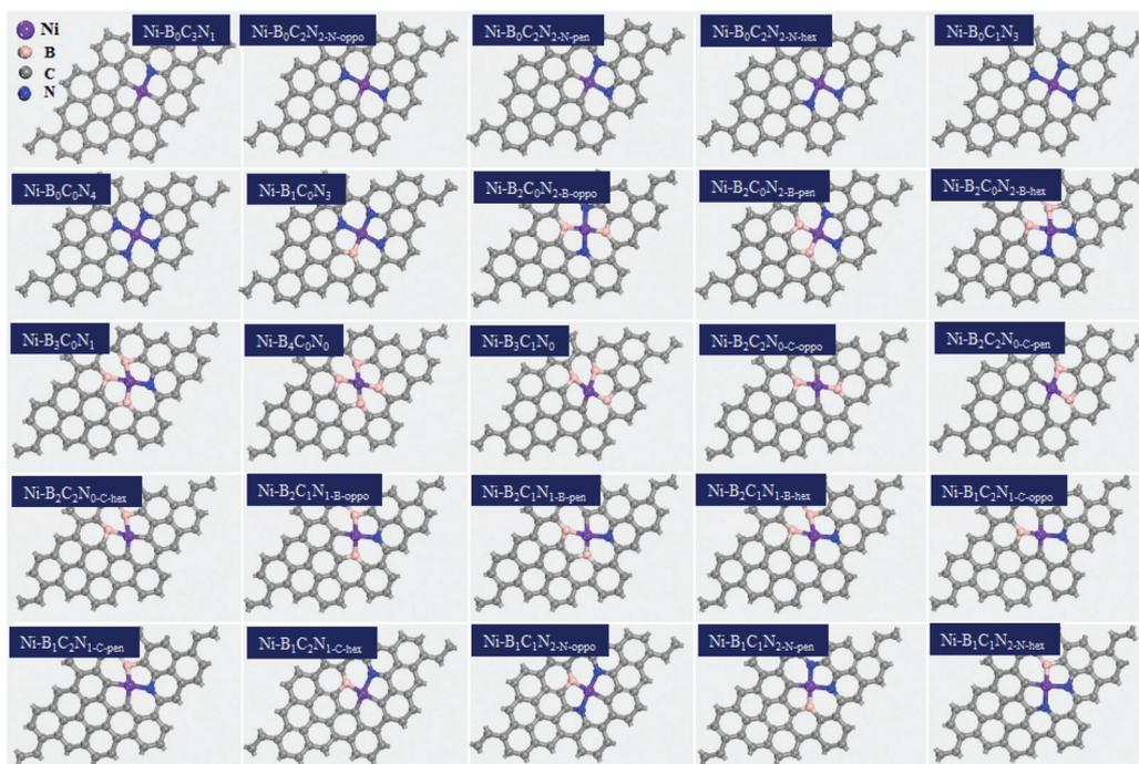
Fig. 2 The optimized structures (top view) of the screened 25 Ni-B<sub>x</sub>C<sub>y</sub>N<sub>z</sub> (X + Y + Z = 4), the color modes: purple for Ni, pink for B, blue for N, and grey for C.
