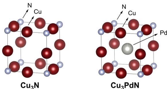
**Fig. 11** Crystal structure of Cu<sub>3</sub>N and the doped Cu<sub>3</sub>PdN. The copper is represented in dark red, the palladium in grey and the nitrogen atom in cyan. Structures plotted using VESTA.<sup>48</sup> Cif file obtained from ref. 111 and 112.
