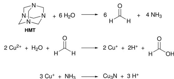
Fig. 17 Proposed reaction mechanism for  $\text{Cu}_3\text{N}$  formation from hexamethylenetetraamine and  $\text{Cu}(\text{NO}_3)_2 \cdot 5\text{H}_2\text{O}$ .<sup>122</sup>
