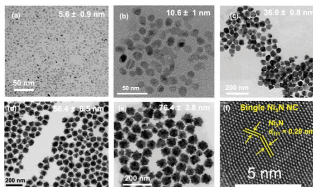
**Fig. 10** TEM images of the different  $\text{Ni}_3\text{N}$  NCs obtained. (a)  $5.6 \pm 0.9$  nm, (b)  $10.6 \pm 1.0$  nm, (c)  $36.6 \pm 0.8$  nm, (d)  $56.4 \pm 6.5$  nm, and (e)  $76.4 \pm 3.8$  nm. (f) High resolution transmission electron microscopy (HRTEM) image of a  $\text{Ni}_3\text{N}$  nanocrystal with a size of  $56.4 \pm 6.5$  nm. Reprinted with permission from ref. 97. Copyright 2021 American Chemical Society.
