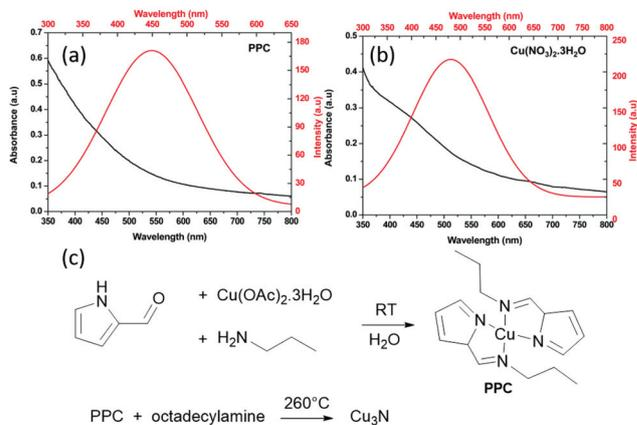
Fig. 18 UV-Vis absorption and photoluminescence spectra of  $\text{Cu}_3\text{N}$  obtained via (a) PPC and (b)  $\text{Cu}(\text{NO}_3)_2 \cdot 3\text{H}_2\text{O}$  method. Reprinted from ref. 124 with permission from the Royal Society of Chemistry. (c) Reaction mechanism proposed for  $\text{Cu}_3\text{N}$  formation from the reaction of pyrrole-2-carbaldpropyliminato Cu(II) (PPC) and ODA shown below.<sup>124</sup>
