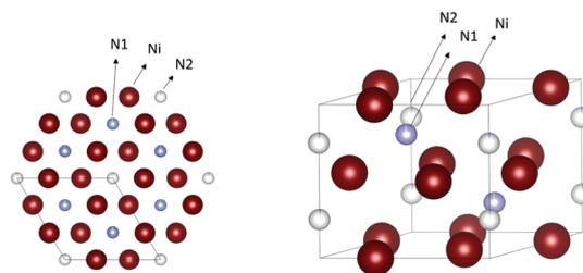
**Fig. 9** Crystal structure of  $\text{Ni}_3\text{N}$ . The nickel atoms are represented in dark red and the nitrogen atoms in cyan and white. Structures plotted using VESTA.<sup>48</sup> Cif file obtained from ref. 89.
