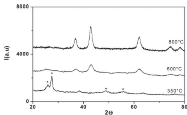
Fig. 7 XRD pattern of titanium-urea gels (*R* = 10) treated at different temperatures. The \* symbol refers to crystalline TiO<sub>2</sub>. Reprinted with permission from ref. 69. Copyright 2009 American Chemical Society.
