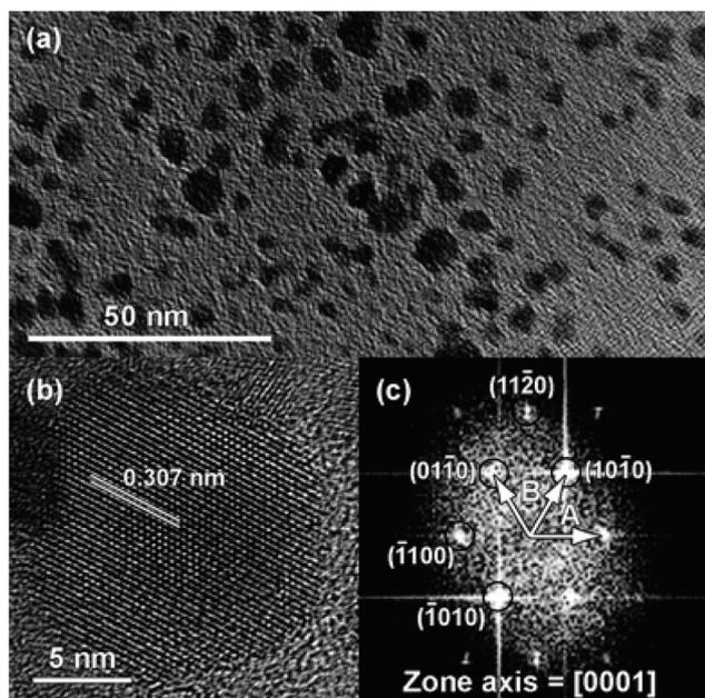
**Fig. 21** TEM images of the colloidal stable InN obtained by Hsieh *et al.* after acid treatment. (a) Low magnification image, (b) high resolution image and (c) diffraction pattern obtained *via* fast Fourier transform (FFT). Reprinted with permission from ref. 173 with permission from the Royal Society of Chemistry.
