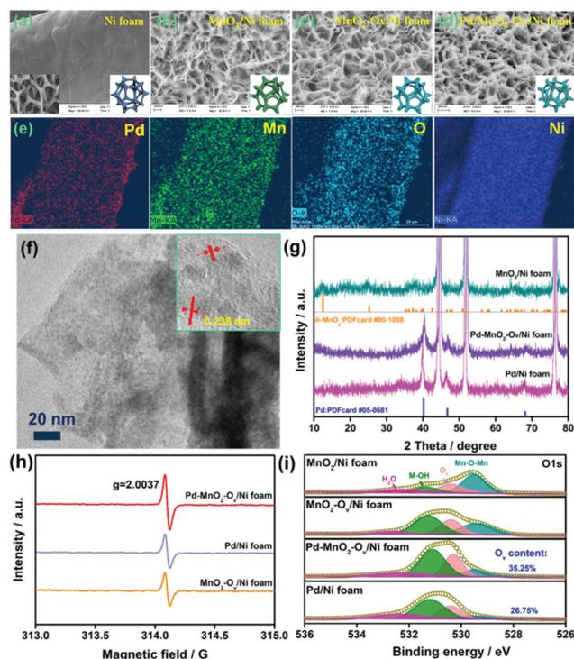
**Fig. 1** Representative SEM images of (a) Ni foam, (b)  $\text{MnO}_2$ /Ni foam, (c)  $\text{MnO}_2\text{-O}_v$ /Ni foam, and (d) Pd– $\text{MnO}_2\text{-O}_v$ /Ni foam; (e) EDS elemental mapping of Pd, Mn, O, and Ni for Pd– $\text{MnO}_2\text{-O}_v$ /Ni foam; (f) TEM image of Pd/ $\text{MnO}_2\text{-O}_v$  nanosheet (inset is the corresponding HRTEM image); (g) XRD patterns of electrodes; (h) EPR spectra and (i) high-resolution O 1s XPS spectra for different electrodes.
