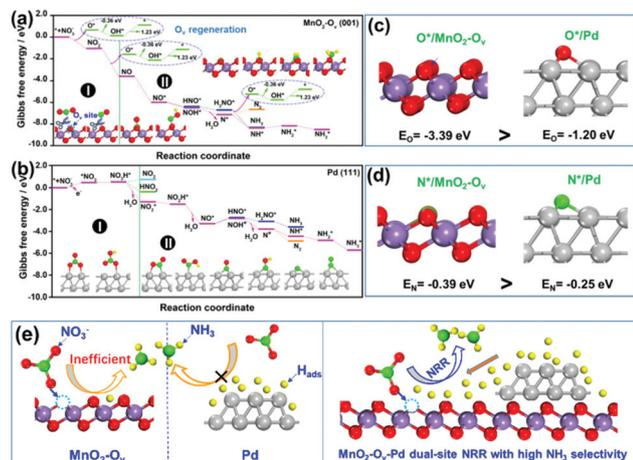
Fig. 4 The reaction energy diagram for the conversion of NO<sub>3</sub><sup>-</sup> to N<sub>2</sub> and NH<sub>3</sub> over (a) clean MnO<sub>2</sub>-O<sub>v</sub> (001) and (b) Pd (111) facet; adsorption energies of (c) one oxygen atom and (d) one nitrogen atom on MnO<sub>2</sub>-O<sub>v</sub> (001) and Pd (111) facets; (e) schematic illustration of the MnO<sub>2</sub>-O<sub>v</sub>-Pd dual-site NRR mechanism for a high NH<sub>3</sub> selectivity.
