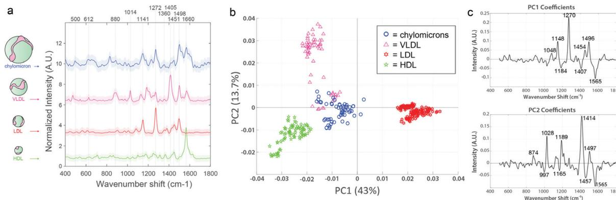
**Fig. 4** Lipoprotein analytical standards are readily distinguished by Raman scattering. (a) SERS spectra of lipoprotein analytical standards, offset for clarity. SERS peaks are readily distinguished from each other. (b) Principal component analysis using PC1 and PC2 (together representing more than 56% of the total variability in the dataset), with loadings (c), shows distinct separation of the lipoprotein subtypes according to spectral differences.
