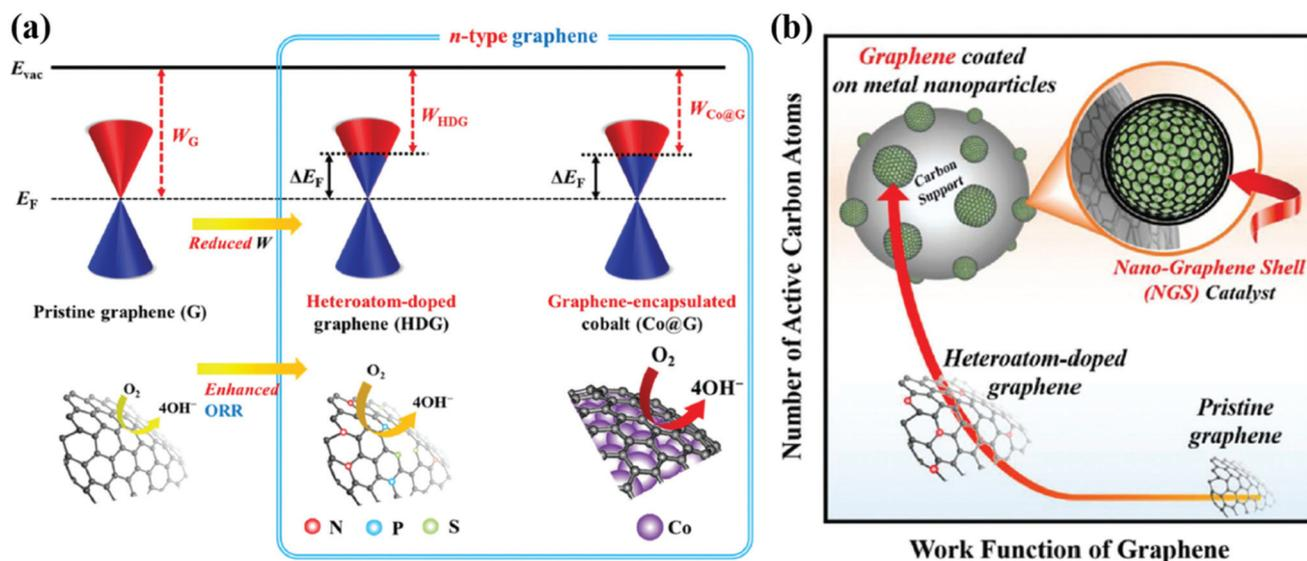
**Fig. 2** Schematic illustration of the electronic effects between the carbon shell and metal nanoparticles (a) Design concept to modify the work function of the carbon shell via Co encapsulation, adapted from ref. 47 with permission from RSC publications, copyright 2019. (b) Advantages of carbon shell encapsulated Pd nanoparticle catalysts, adapted from ref. 48 with permission from RSC publications, copyright 2019.
