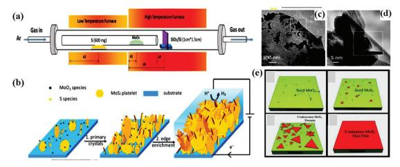
Fig. 3 (a) Schematic representation showing the experimental CVD setup, (b) mechanistic demonstration of the edge enrichment of MoS<sub>2</sub>, (c) and (d) TEM images of the petal site showing the nucleation of vertically aligned nanoflakes on the top-layer crystals. Reproduced from ref. 85. (e) Schematic illustration of monolayer MoS<sub>2</sub> growth on a Piranha-treated substrate. Reproduced from ref. 86.
