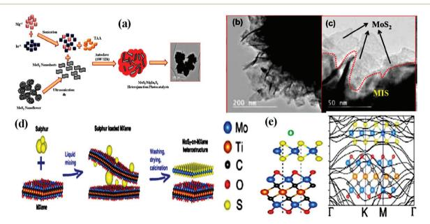
Fig. 6 (a) Schematic diagram showing the growth mechanism and (b) and (c) corresponding HRTEM images of MoS<sub>2</sub>/MgIn<sub>2</sub>S<sub>4</sub> heterojunction photocatalyst. Reproduced with permission. 90 (d) Schematic representation of the fabrication of MoS<sub>2</sub>/MXene hybrids and (e) structural stacking patterns and electronic band structure of MoS<sub>2</sub>/Mo<sub>2</sub>TiC<sub>2</sub>O<sub>2</sub>. Reproduced with permission.<sup>105</sup>
