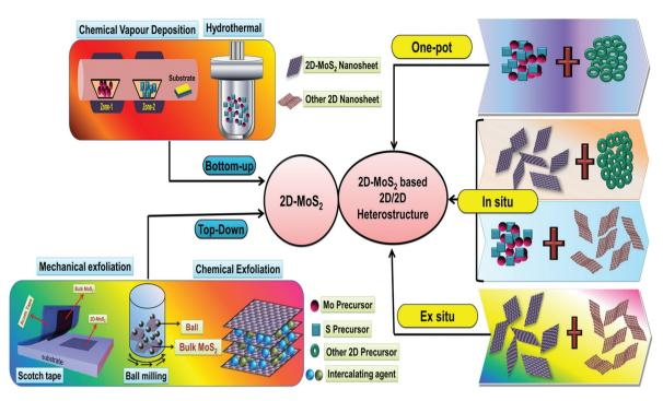
Scheme 2 Schematic illustration of the various techniques used for the synthesis of 2D-MoS<sub>2</sub> and its 2D/2D-heterostructures.
