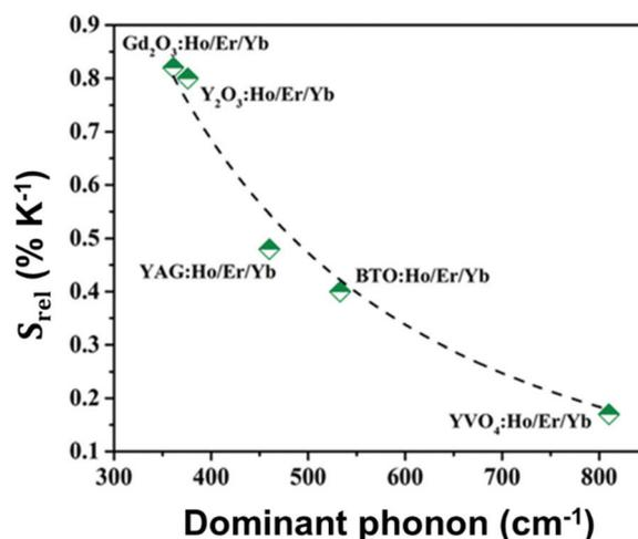
**Fig. 36**  $S_{rel}$  of  $Er^{3+}, Ho^{3+}, Yb^{3+}$ -co-doped nanoparticles as a function of the dominant phonon energy. Reprinted with permission from ref. 254. Copyright 2020, Wiley-VCH Verlag GmbH & Co. KGaA.
