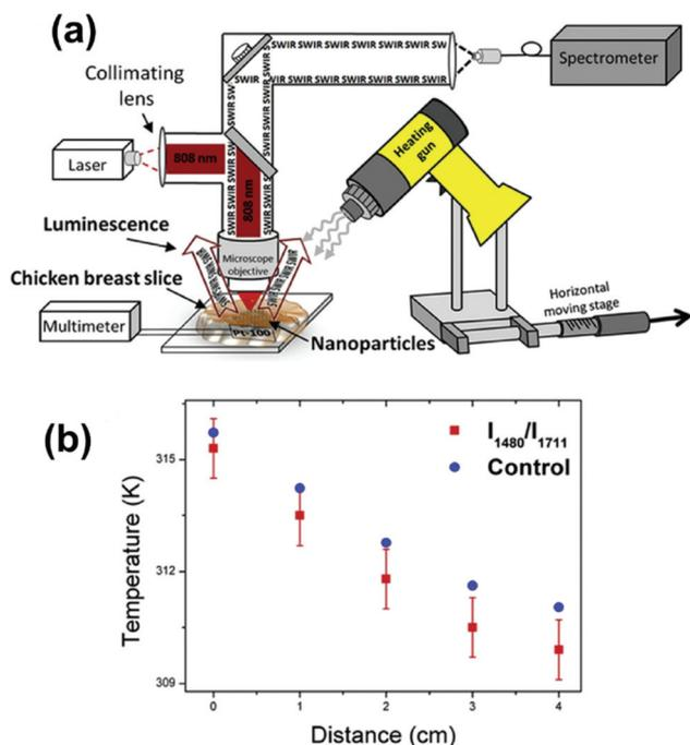
**Fig. 47** *Ex vivo* temperature sensing in the III-BW with Ho, Tm:KLu( $\text{WO}_4$ )<sub>2</sub> nanoparticles. (a) Schematic representation of the experimental setup. (b) Temperature profile determined from the intensity ratio of the 1480 nm and 1711 nm emission bands of  $\text{Tm}^{3+}$  in Ho,Tm:KLu( $\text{WO}_4$ )<sub>2</sub> particles (red squares) and by a Pt-100 thermocouple (blue spheres). Reprinted with permission from ref. 265. Copyright 2018, Elsevier.
