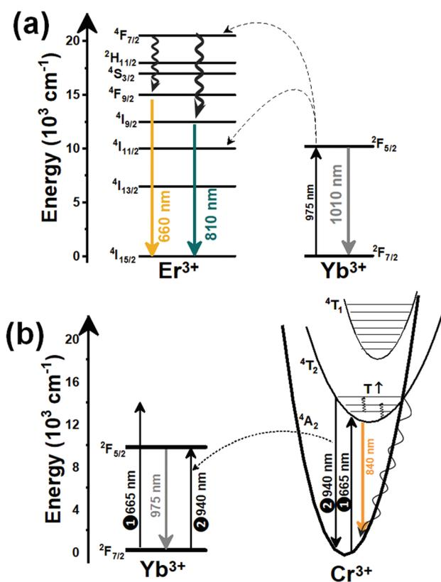
Fig. 24 Mechanisms of generation of the emission lines of dual-doped (a)  $\text{Er}^{3+}/\text{Yb}^{3+}$  and (b)  $\text{Cr}^{3+}/\text{Yb}^{3+}$  materials operating simultaneously in the I- and II-BWs.
