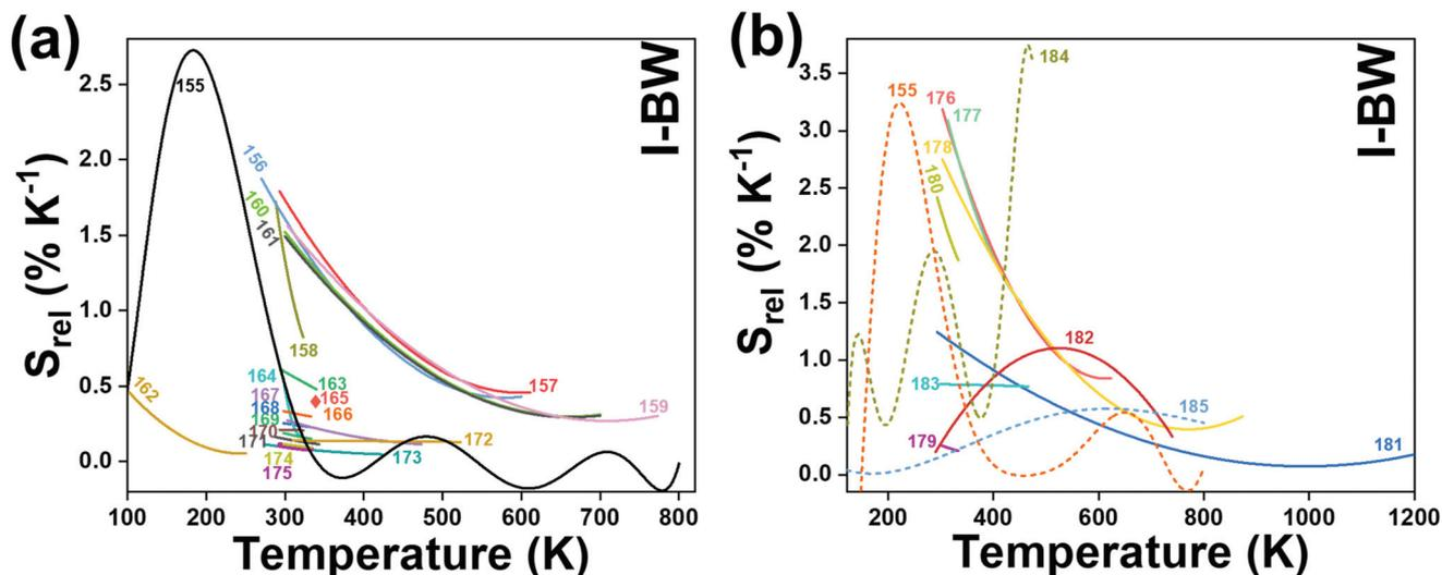
Fig. 15 Temperature dependence of  $S_{rel}$  for: (a) single doping and (b) codoping with other lanthanide ions (in solid lines) and transition metal ions (in dashed lines) for Nd<sup>3+</sup> luminescent thermometers, operating in the I-BW. The numbers represent the corresponding references for each Nd<sup>3+</sup>-based thermometer.
