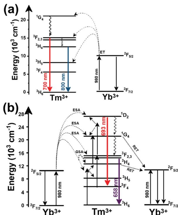
**Fig. 6** Mechanisms of generation of the emission lines for: (a)  $\text{Tm}^{3+}, \text{Yb}^{3+}:\text{GdVO}_4@\text{SiO}_2$  core@shell nanoparticles (as an illustrative example) after excitation at 980 nm, and (b)  $\text{Tm}^{3+}, \text{Yb}^{3+}$ -doped phosphate glass material after excitation at 980 nm.
