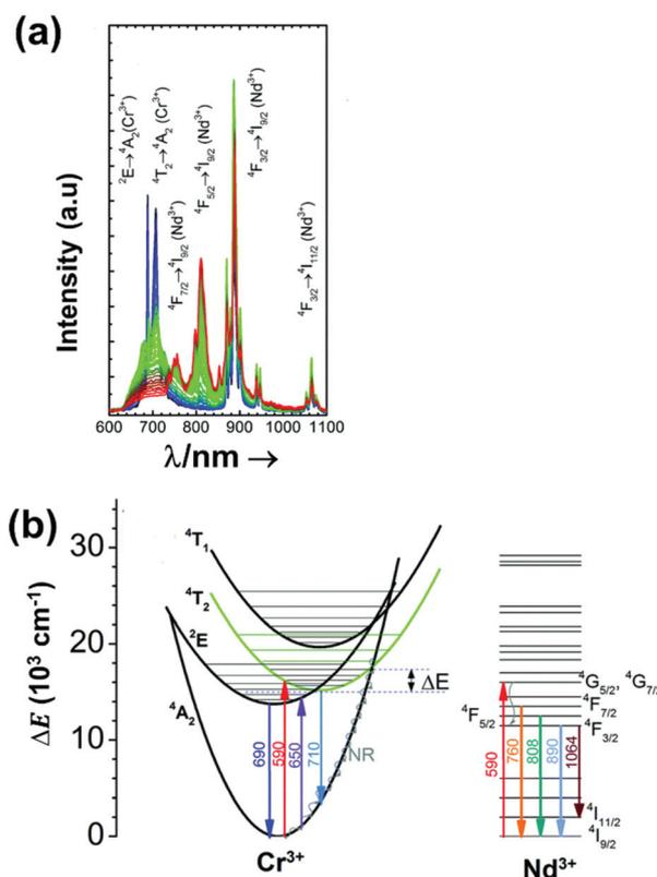
Fig. 16 (a) Emission lines and (b) mechanisms for their generation in Nd<sup>3+</sup>,Cr<sup>3+</sup>-codoped YAG, after being excited at 590 nm. Reprinted with permission from ref. 155. Copyright 2017, the Owner Societies.
