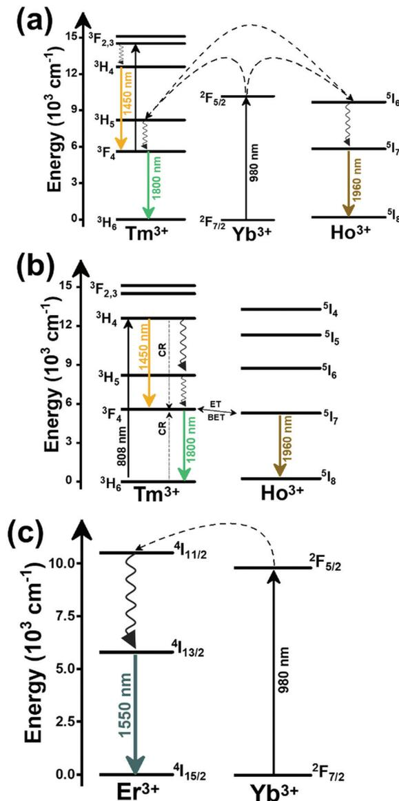
Fig. 40 Mechanism of the generation of the emission lines in: (a)  $\text{Ho}^{3+}, \text{Tm}^{3+}, \text{Yb}^{3+}:\text{KLu}(\text{WO}_4)_2$ , (b)  $\text{Ho}^{3+}, \text{Tm}^{3+}:\text{KLu}(\text{WO}_4)_2$ , and (c)  $\text{Er}^{3+}, \text{Yb}^{3+}$ -doped materials operating as luminescent thermometers in the III-BW.
