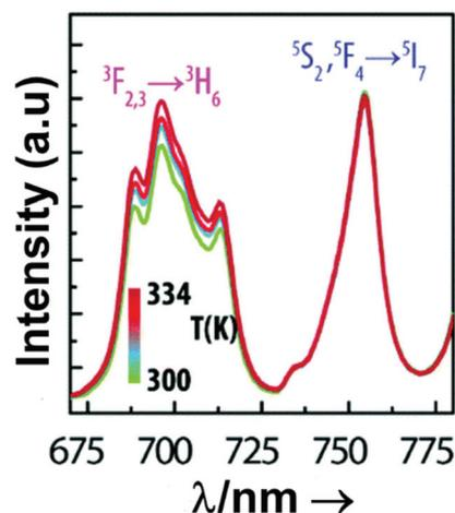
Fig. 10 Temperature dependence of the emission spectra of Ho,Tm:KLu(WO<sub>4</sub>)<sub>2</sub> nanocrystals, demonstrating the similar intensity between the  ${}^3\text{F}_{2,3} \rightarrow {}^3\text{H}_6$  of  $\text{Tm}^{3+}$  and  ${}^5\text{S}_2, {}^5\text{F}_4 \rightarrow {}^5\text{I}_7$  of  $\text{Ho}^{3+}$ . Reprinted with permission from ref. 150. Copyright 2018, The Royal Society of Chemistry.
