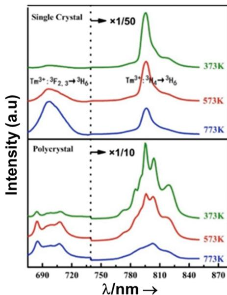
**Fig. 8** Emission spectra of  $\text{Tm}^{3+}/\text{Yb}^{3+}$ -codoped  $\text{LiNbO}_3$  polycrystal and single crystal at different temperatures under 980 nm excitation (1/10 and 1/50 represent the factor of division applied above the marked wavelength to visualize clear the different emission bands). Reprinted with permission from ref. 133. Copyright 2015, Elsevier.
