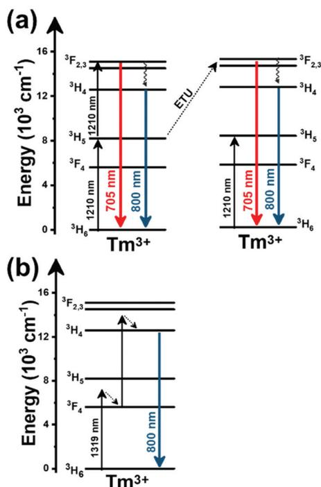
**Fig. 5** Mechanisms of generation of the emission lines for single active Tm<sup>3+</sup>-doped luminescent thermometers: (a) YAP after excitation at 1210 nm and (b) NaNbO<sub>3</sub> after excitation at 1319 nm. Please note that despite the fact that other emission lines can be produced, for sake of simplicity, only the emission lines involved in the luminescence thermometer development are considered.
