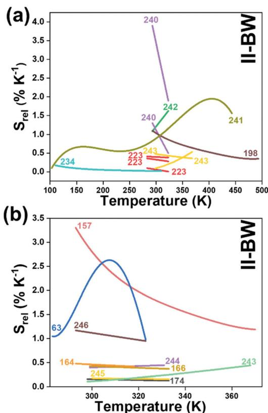
Fig. 32 Temperature dependence of  $S_{\text{rel}}$  of: (a)  $\text{Yb}^{3+}$ - and (b)  $\text{Nd}^{3+}$ -doped luminescent thermometers operating in the II-BW region. The numbers indicate corresponding references for each thermometer.
