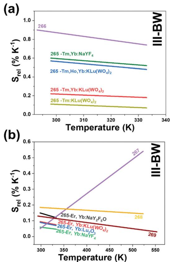
Fig. 43 Temperature dependence of  $S_{rel}$  of: (a) Tm<sup>3+</sup>- and (b) Er<sup>3+</sup>-doped thermometers operating in the III-BW. The numbers indicate the corresponding references for each thermometer.
