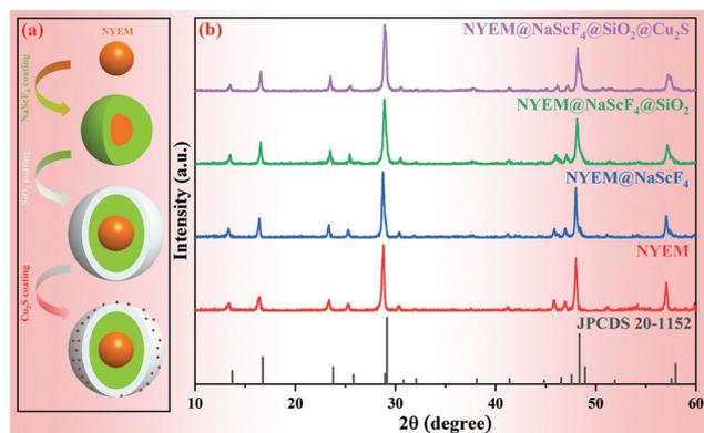
**Fig. 1** (a) A description of the preparation of  $\text{NYEM@NaScF}_4\text{@SiO}_2\text{@Cu}_2\text{S}$ . (b) XRD diffraction patterns of the samples synthesized at various steps along with the reference data of hexagonal  $\text{NaScF}_4$  (JCPDS 20-1152).
