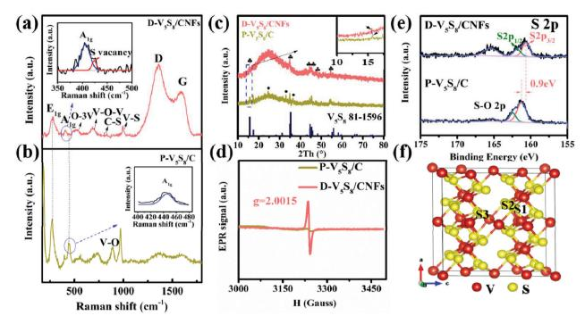
Fig. 2 (a and b) Raman spectra, (c) XRD pattern, (d) EPR spectrum, and (e) XPS analysis of the  $P-V_5S_8/C$  and  $D-V_5S_8/CNF$  samples. (f) Schematic illustration of the atom arrangements in  $V_5S_8$ ; note that S1, S2, and S3 represent the possible sulfur defects.
